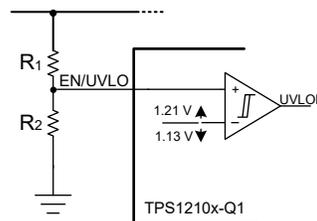
**Figure 9-10. Programming Undervoltage Protection**
