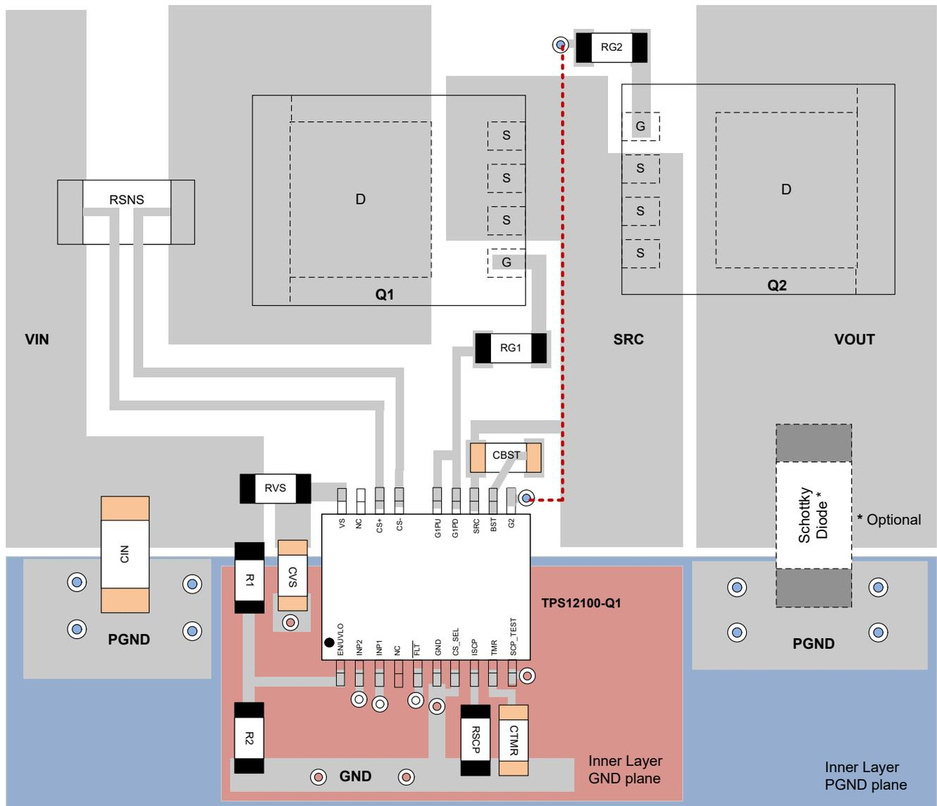
**Figure 10-12. Typical PCB Layout Example for TPS1210-Q1 With B2B MOSFETs**
