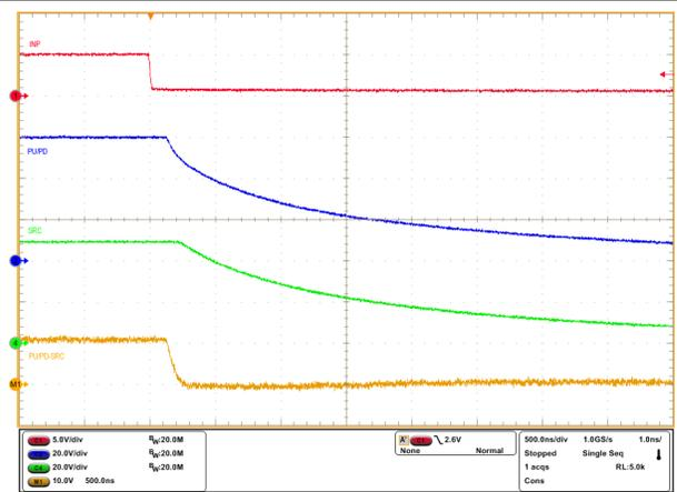
Figure 10-5. Turn-OFF Response of TPS12100-Q1 for INP1 -> HIGH to LOW and  $C_{BST} = 470$  nF
