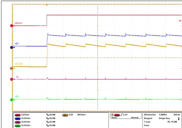
Figure 10-2. Start-Up Profile of Bootstrap Voltage with INP1=INP2 = GND and  $C_{BST} = 470$  nF
