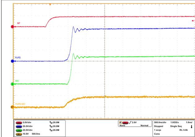
Figure 10-4. Turn-ON Response of TPS12100-Q1 for INP1 -> LOW to HIGH and  $C_{BST} = 470$  nF
