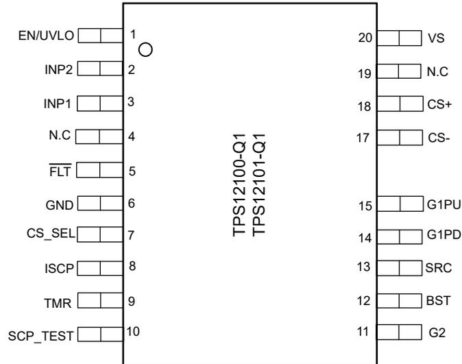
Figure 6-1. VSSOP 19-Pin DGX Top View
