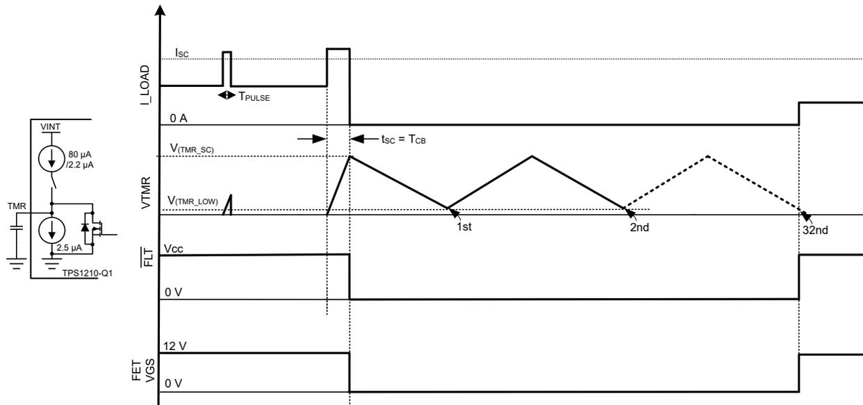
Figure 9-8. Short-Circuit Protection With Auto-Retry
