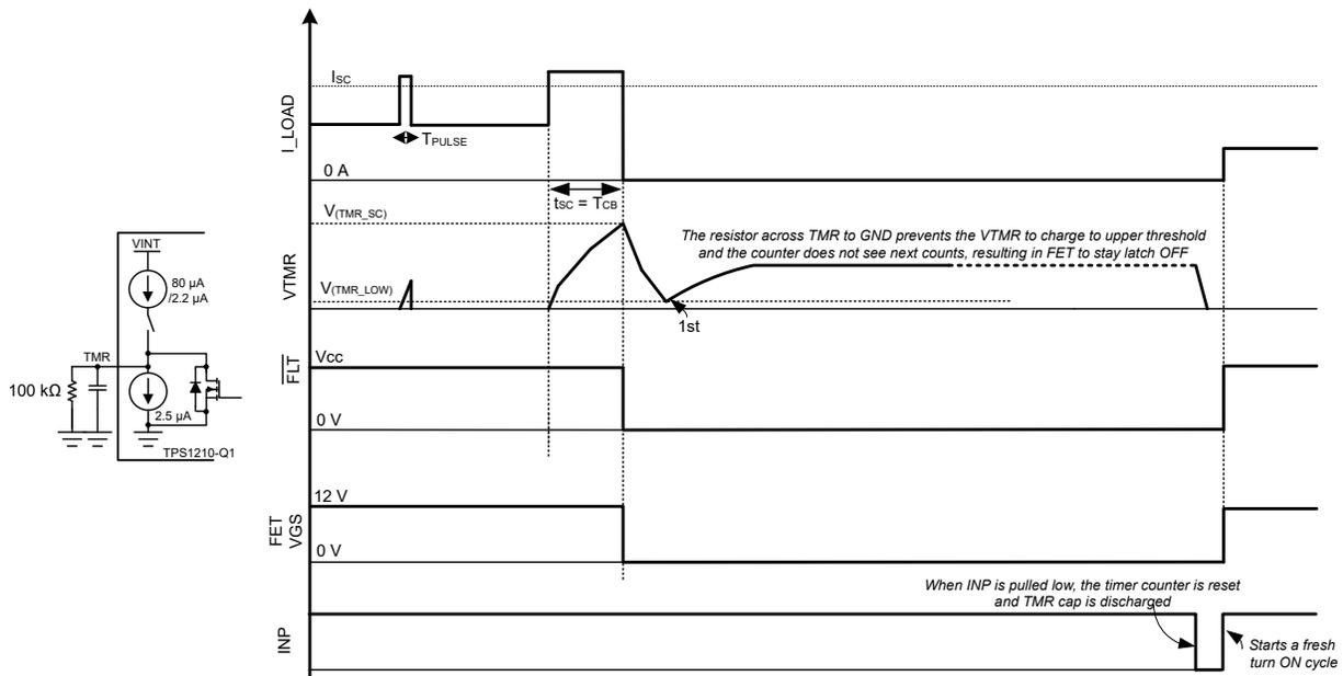
**Figure 9-9. Short-Circuit Protection With Latch-Off**
