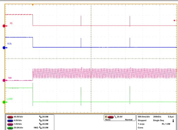
Figure 10-7. Auto-Retry Response of TPS12100-Q1 for an Overcurrent Fault
