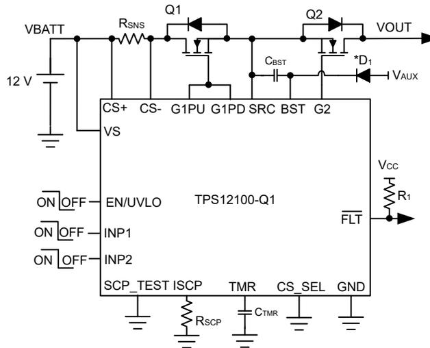
Figure 9-3. TPS1210-Q1 Application Circuit With External Supply to BST
