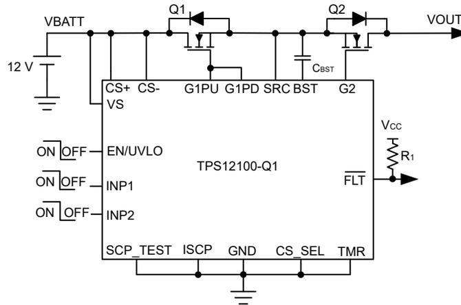
Figure 9-11. TPS1210-Q1 Application Circuit for Simple Gate Driver
