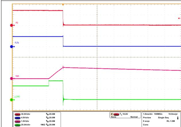
Figure 10-6. Overcurrent Response of TPS12100-Q1 for a Load Step from 25 A to 35 A with 30-A Overcurrent Protection Setting
