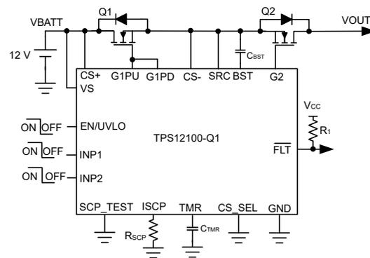
Figure 9-6. TPS1210-Q1 Application Circuit With MOSFET RDSON based Current Sensing
