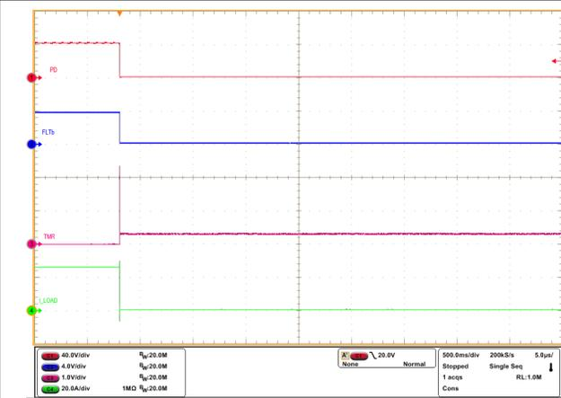
**Figure 10-8. Latch-Off Response of TPS1210-Q1 for an Overcurrent Fault**
