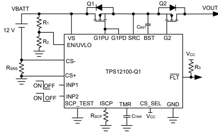
Figure 10-1. Typical Application Schematic: BMS Circuit Breaker With Low Side Current Sense
