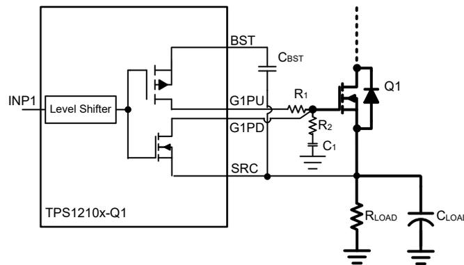
Figure 9-4. Inrush Current Limiting Using G1 Gate Drive
