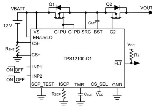
**Figure 9-7. TPS1210-Q1 Application Circuit with External Sense Resistor RSNS based Low Side Current Sensing**
