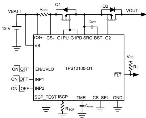
Figure 9-5. TPS1210-Q1 Application Circuit With External Sense Resistor  $R_{SNS}$  based High Side Current Sensing
