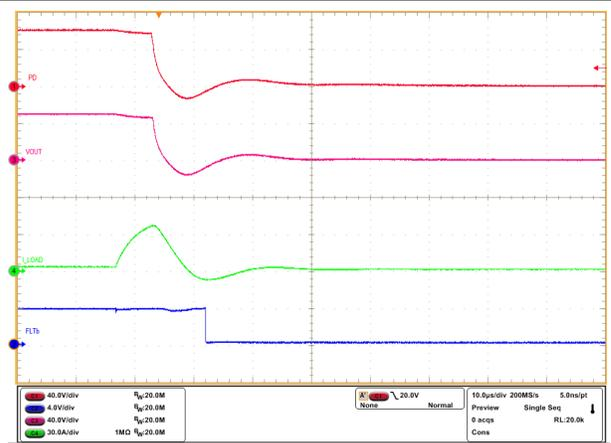
**Figure 10-9. Output Short-Circuit Response of TPS1210-Q1 Device**
