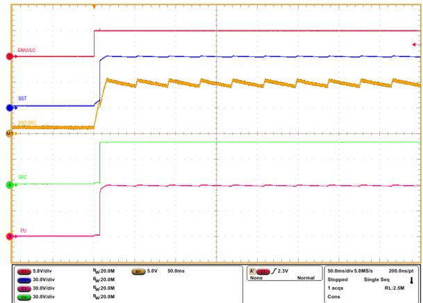
Figure 10-3. Start-Up Profile of Bootstrap Voltage with INP1=INP2 = HIGH and  $C_{BST} = 470$  nF
