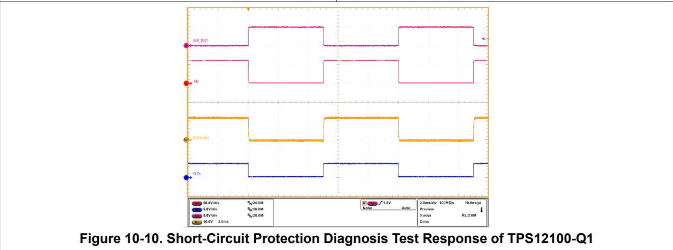
**Figure 10-10. Short-Circuit Protection Diagnosis Test Response of TPS1210-Q1**
