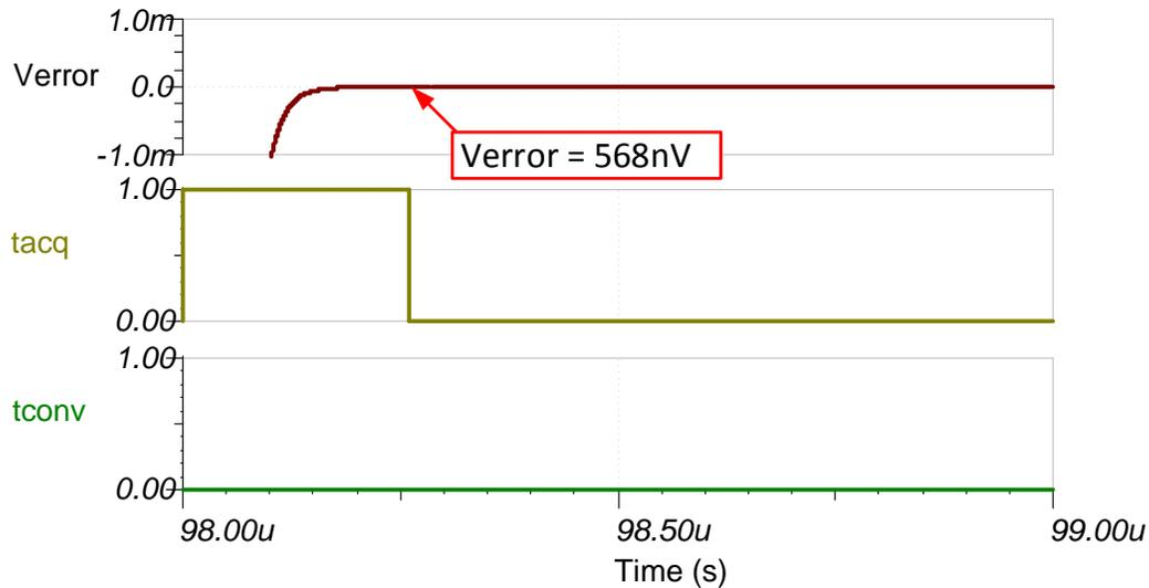
**Transient ADC Input Settling Simulation Lower Sampling rate – 200ksps on ADS8568+OPA192**
