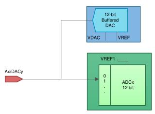
Figure 6-7. DAC to ADC Loopback
