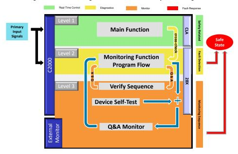
Figure 4-4. VDA E-Gas Monitoring Concept Applied to F28003x MCU
