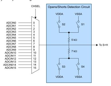
Figure 6-8. ADC Open-Shorts Detection Circuit
