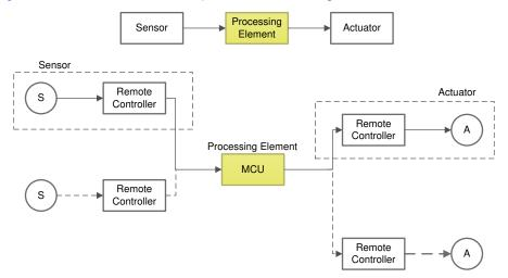
Figure 4-2. Definition of the TMS320F28003x MCU Used in a Compliant Item
