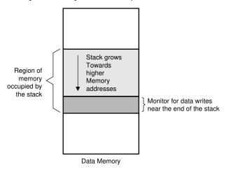
Figure 6-2. Stack Overflow Monitoring
