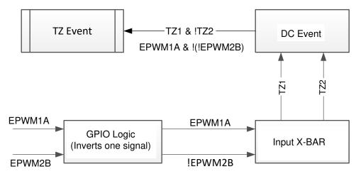
Figure 6-3. ePWM Fault Detection Using X-BAR
