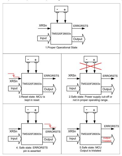
Figure 4-8. TMS320F28003x MCU Safe State Definition
