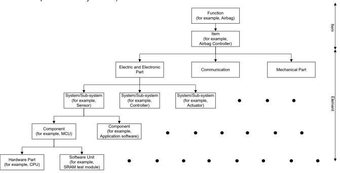
Figure C-1. ISO 26262 Illustration of Item, System, Component, Hardware Part and Software Unit
