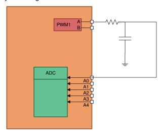
Figure 6-4. Monitoring of ePWM by ADC
