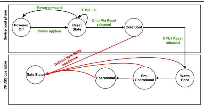
Figure 4-9. TMS320F28003x MCU Device Operating States
