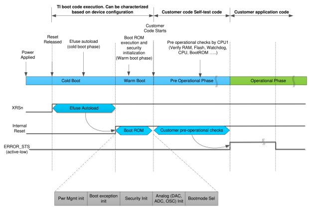
Figure 4-10. TMS320F28003x MCU CPU Start-Up Sequence
