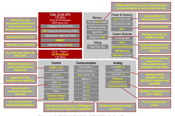
Figure 4-5. TMS320F28003x MCU With Safety Features
