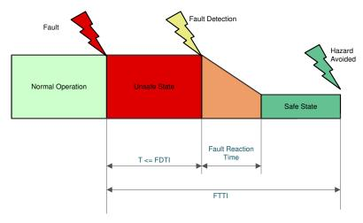
Figure 4-6. Relationship Between FDTI, Fault Reaction Time and FTTI
