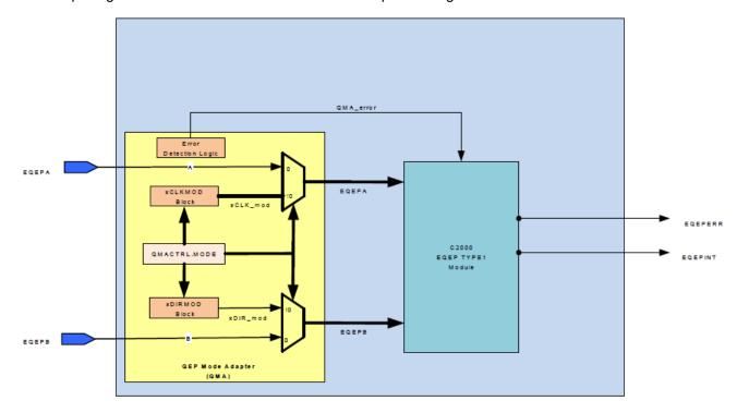
Figure 6-6. QMA Module Block Diagram
