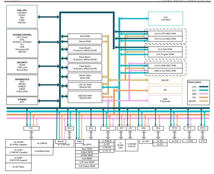
Figure 4-1. Functional Block Diagram of TMS320F28003x MCU
