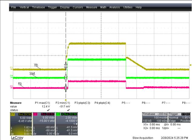
Figure 3-10. Start-Up Shut-Down,  $V_{OUT} = 3.3V$
