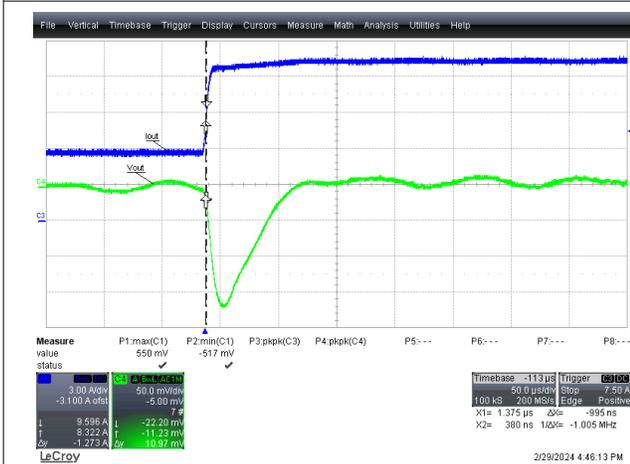
Figure 3-11. Load Transient Rising,  $V_{OUT} = 5V$ ,  $I_{OUT} = 6A$  to  $12A$
