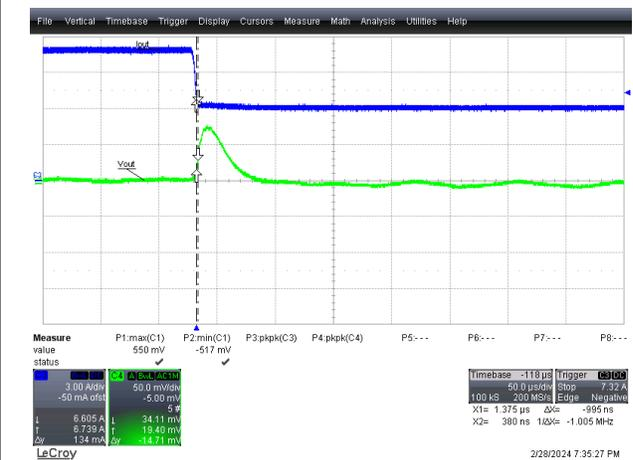
Figure 3-14. Load Transient Falling,  $V_{OUT} = 3.3V$ ,  $I_{OUT} = 12A$  to  $6A$
