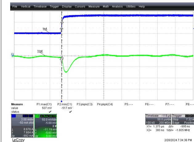
Figure 3-13. Load Transient Rising,  $V_{OUT} = 3.3V$ ,  $I_{OUT} = 6A$  to  $12A$
