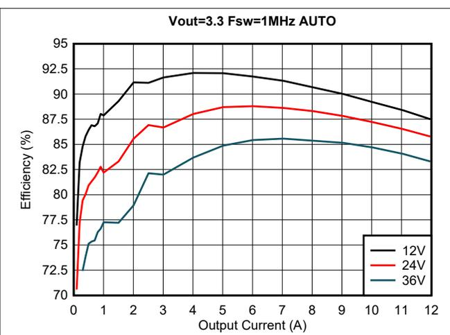
Figure 3-2. Efficiency, VOUT = 3.3V, AUTO Mode
