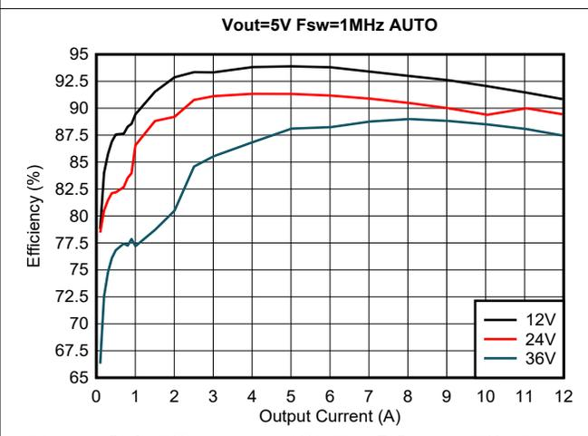
Figure 3-4. Efficiency, VOUT = 5.0V, AUTO Mode
