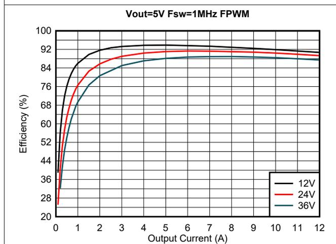
Figure 3-3. Efficiency, VOUT = 5.0V, FPWM Mode
