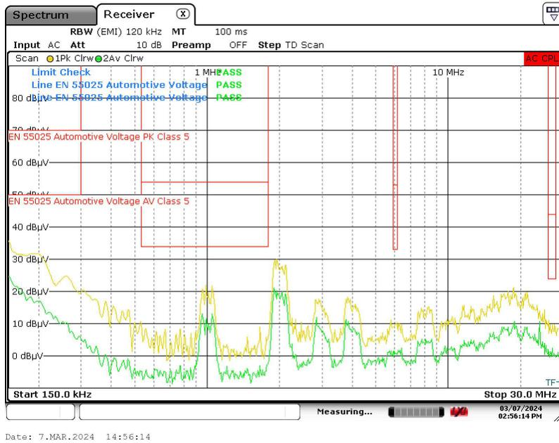
Figure 3-17. CISPR 25 Conducted Emissions: 150kHz to 30MHz
