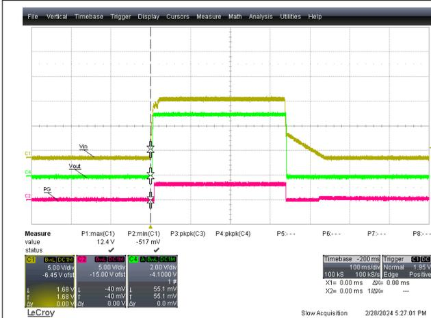
Figure 3-9. Start-Up Shut-Down,  $V_{OUT} = 5V$
