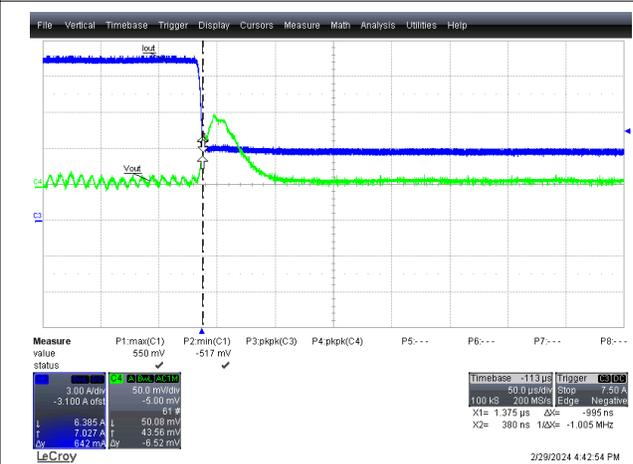
Figure 3-12. Load Transient Falling,  $V_{OUT} = 5V$ ,  $I_{OUT} = 12A$  to  $6A$
