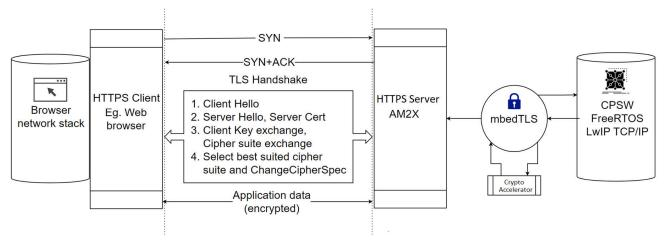
Figure 3-2. Overview of How HTTPS Server Example Works End to End
