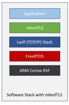
Figure 2-1. MbedTLS Secure Communication Over TCP/IP Stack
