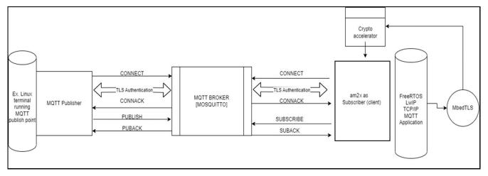
Figure 3-3. Overview of Working of MQTT + TLS Client
