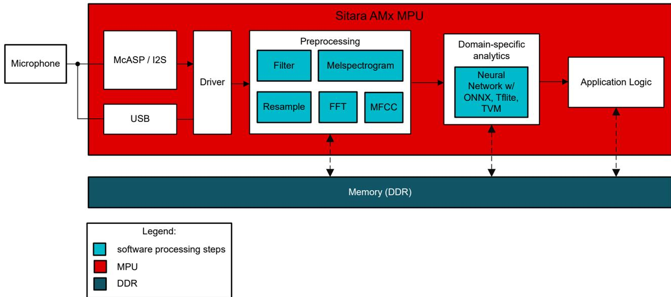
**Figure 1. Block Diagram of Audio Processing Flow for a Keyword Spotting Application Using Neural Networks on AMx MPUs**
