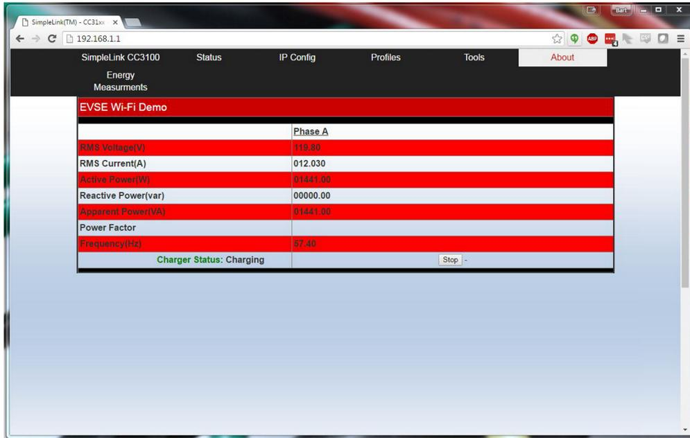
Figure 33. EVSE Web Page Showing Charging State
