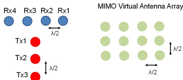
**Figure 2-3. AWR1843AOP-Antenna Pattern**
