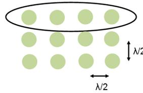
**Figure 2-6. Virtual Antenna Array for Range-Azimuth-Angle Heat-Map Calculation**
