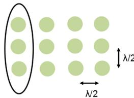
Figure 2-5. Virtual Antenna Array for Range-Elevation-Angle Heat-Map Calculation
