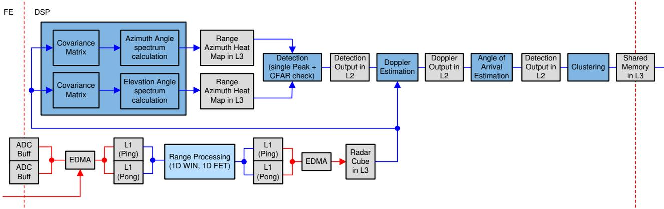
Figure 2-4. System Process Chain
