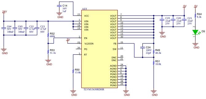
Figure 3-3. 5-V Regulator Schematic
