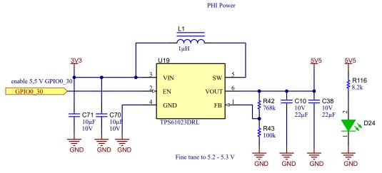
Figure 3-5. 5.5-V Boost Regulator Schematic
