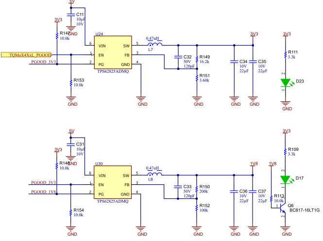
Figure 3-4. 3.3-V and 1.8-V Regulator Schematic
