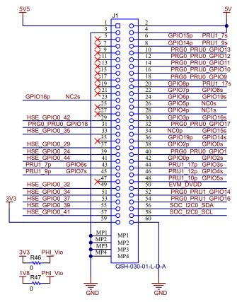
Figure 3-9. PHI Header Pinout
