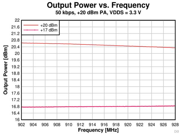
**Figure 8-27. Output Power vs. Frequency (50 kbps, 915 MHz, VDDS = 3.3 V)**
