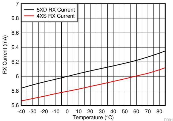
Figure 8-12. RX Mode Current Consumption vs Temperature D001
