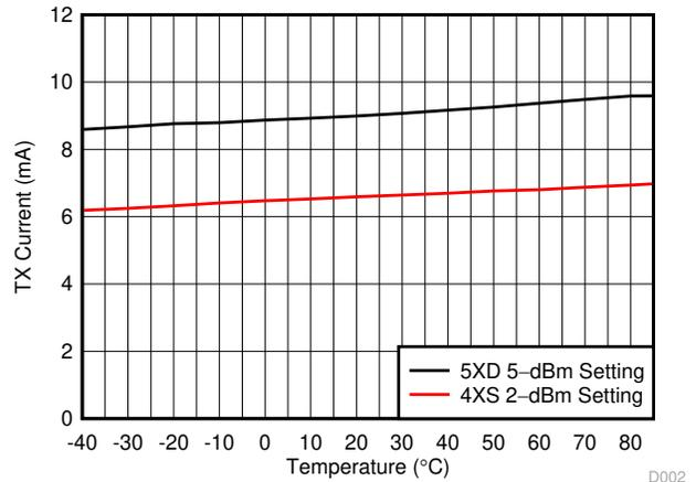
Figure 8-13. TX Mode Current Consumption vs Temperature D002
