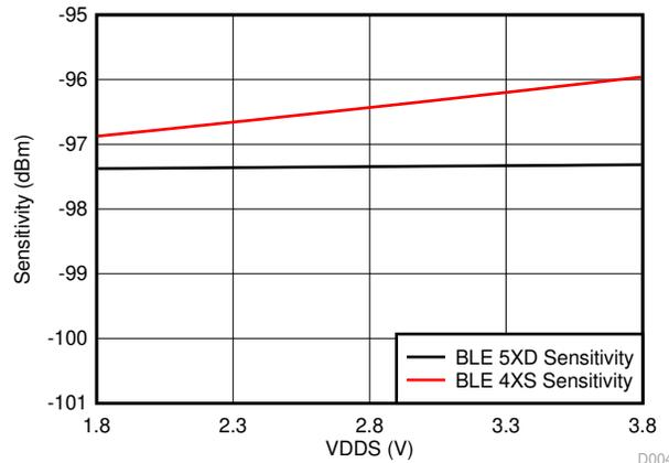
Figure 8-5. BLE Sensitivity vs Supply Voltage (VDD5)
