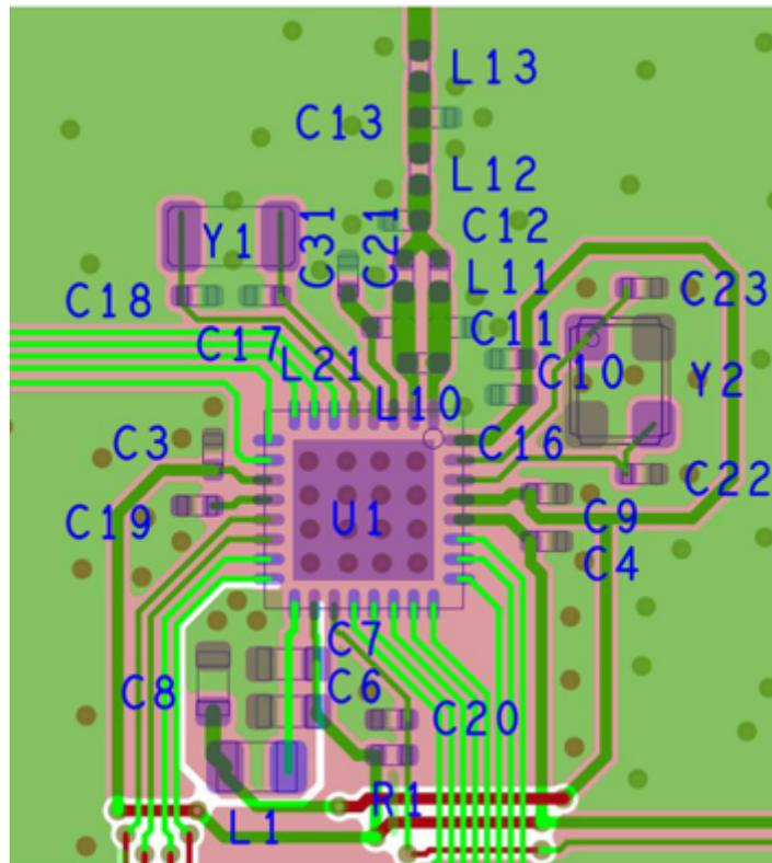
Figure 10-4. 5 × 5 External Differential (5XD) Layout
