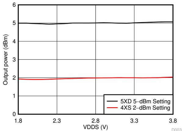
Figure 8-8. TX Output Power vs Supply Voltage (VDD5)
