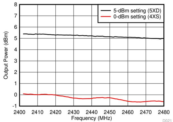
Figure 8-9. TX Output Power vs Channel Frequency
