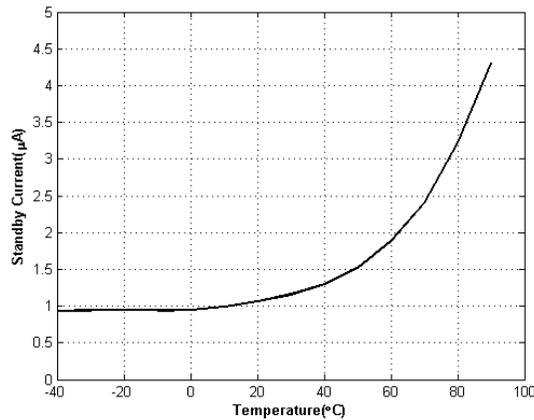
**Figure 8-20. Standby Mode Supply Current vs Temperature**
