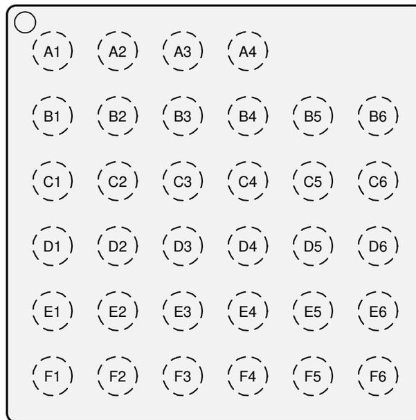
Figure 7-3. YFV (2.7-mm × 2.7-mm) Pinout, Top View
