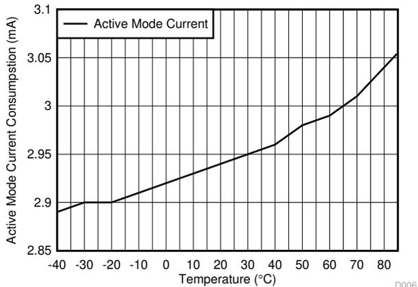
Figure 8-14. Active Mode (MCU Running, No Peripherals) Current Consumption vs Temperature D006
