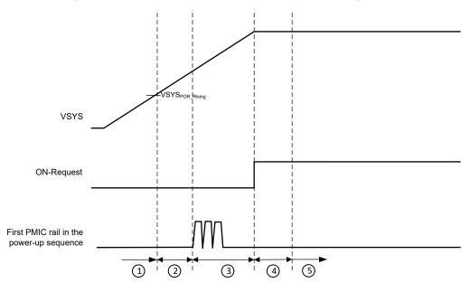
Figure 6-1. VSYS Slow Ramp with FSD Enabled
