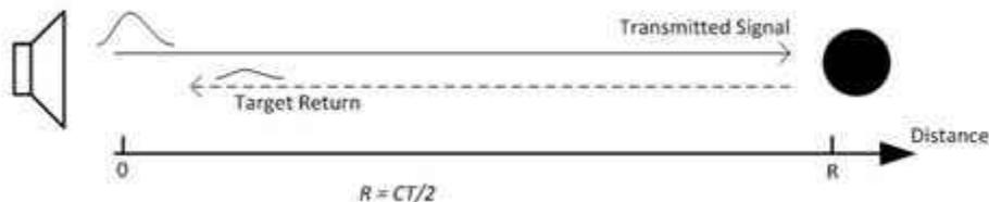
**Figure 1. Sonar Used in Target-range Measurement**
