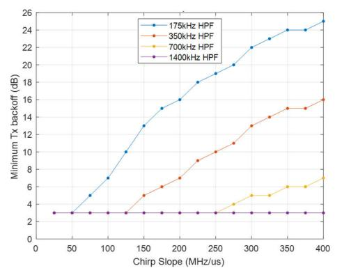
Figure 4-2. Minimum TX Backoff for 57 to 64GHz
