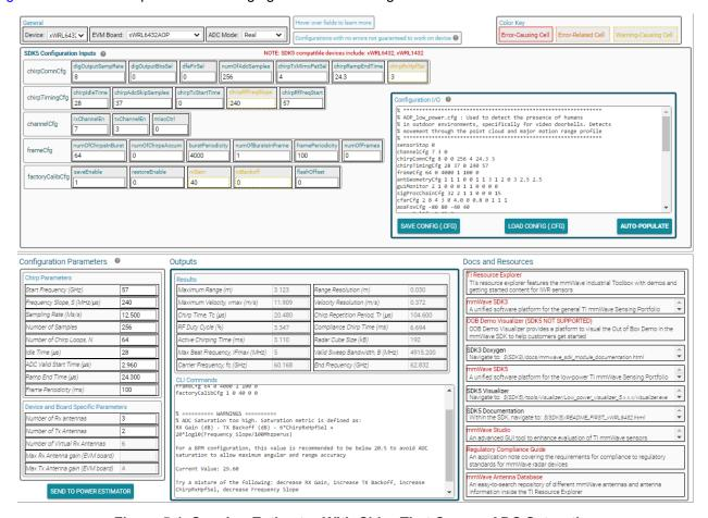
Figure 5-1. Sensing Estimator With Chirp That Causes ADC Saturation
