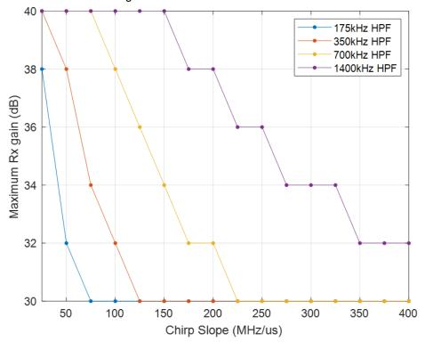
Figure 4-1. Maximum Allowed RX Gain Setting
