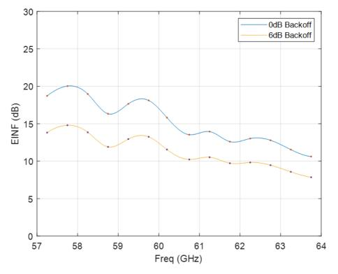
Figure 2-2. Average EINF With Single TX on Across Frequencies
