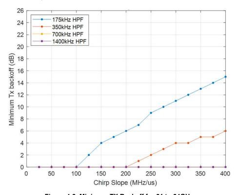
Figure 4-3. Minimum TX Backoff for 61 to 64GHz
