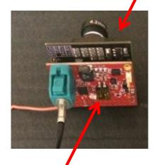
Serializer Board with power (used for test)
