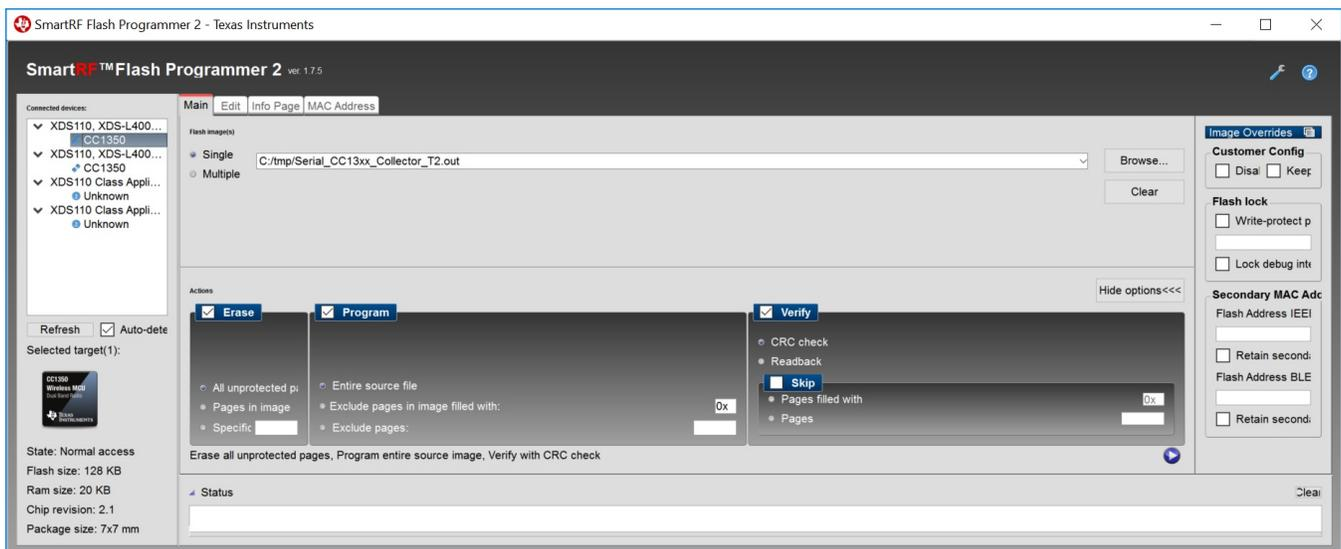
**Figure 4. TI wM-Bus Stack (Data Collector Binary) Programming of CC1350 LaunchPad**
