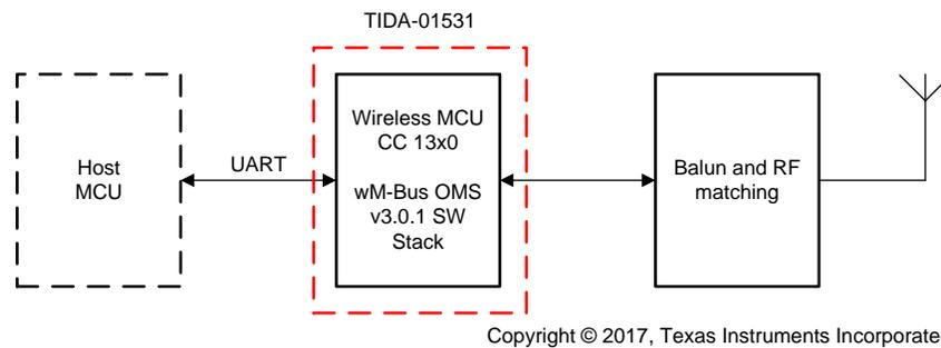
**Figure 1. TIDA-01531 Block Diagram**
