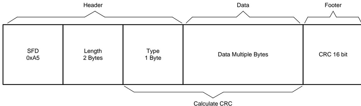
**Figure 17. Commands Format Used in Serial Version of TI wM-Bus Stack (by STACKFORCE GmbH)**
