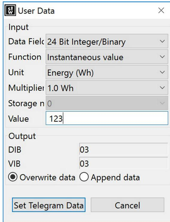
**Figure 14. Modified "123" Energy Value for Meter Data Packet**
