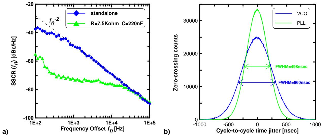
Fig. 5. a) Experimental SSCR curves for the LC-tuned VCO and PLL built around it. The discrepancy with the pure  $1/f^2$  trend of the VCO plot is due to a residual PLL action. b) Statistical distributions of the period duration as collected at the MCA of the setup in Fig. 4
