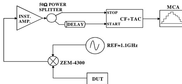
**Fig. 4.** Block diagram of the lab setup. A low-noise instrumentation amplifier can provide for image rejection, whereas the coaxial stub is used to synchronize the operation of the zero-crossing detector [3]
