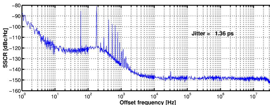
Fig. 9.  $SSCR$  vs.  $f_n$  offset frequency profile of the external source at 30MHz, as obtained from the Aeroflex PN9000 phase noise analyzer
