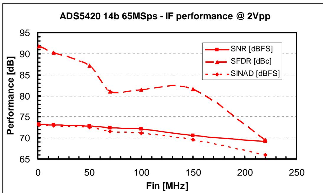
Fig. 10.  $f_{in}$  sweep at 65MSps sampling rate on TI's ADS5420 14 bit 65MSps A-to-D converter for wireless infrastructure applications
