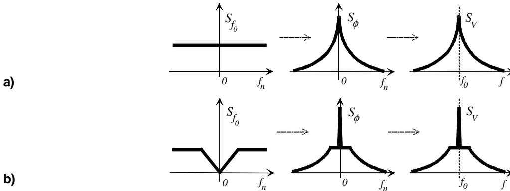
**Fig. 1.** Power spectral densities of frequency noise, phase noise, and output voltage noise in the case of a) a free-running oscillator, b) a PLL frequency synthesizer
