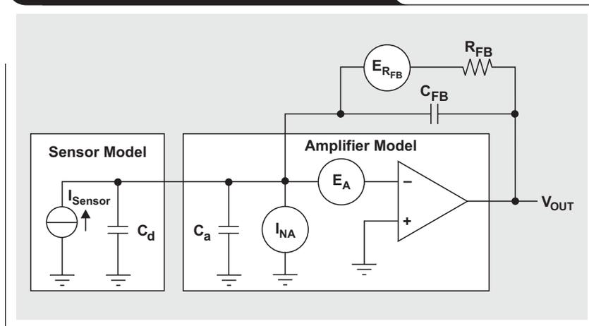
**Figure 5. OPA337's input-voltage and input-current noise**
