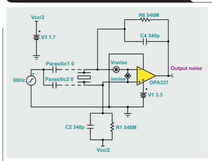
**Figure 18. Differential amplifier nearly eliminates common-mode noise**
