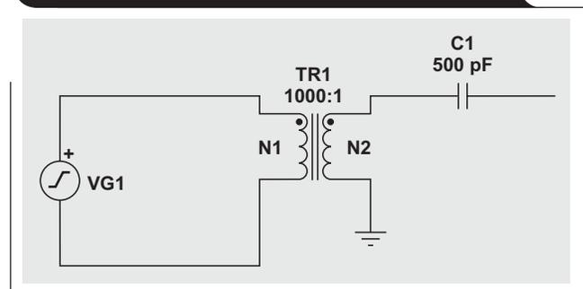
0.5 pC/g and a parasitic capacitance of 500 pF is modeled. The sinusoidal generator outputs 1 V for every unit of g to be simulated. The transformer scales that down to 1 mV on its secondary. A 1-mV swing applied to C1 (500 pF) would inject  $Q = VC = 0.5$  pC on the next stage, as expected.
