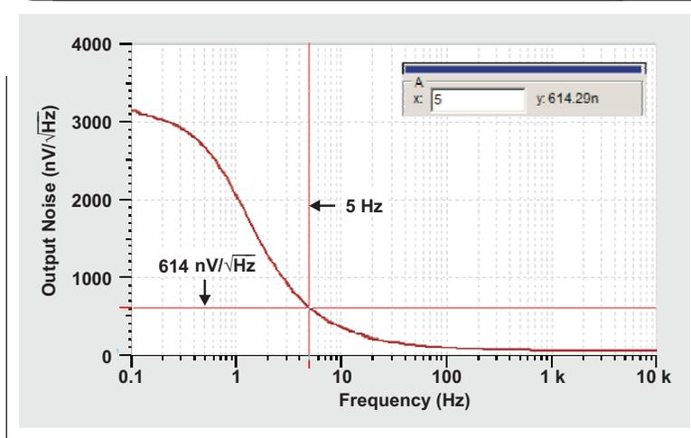
close to the simulation result (see Figure 14). As expected, the output noise goes up. Nevertheless, doubling the resistance allows the capacitance to be divided by two, effectively doubling the gain (i.e., doubling the output signal). Even though  $R_{FB}$  is the dominant noise source, and increasing it increases its noise, an SNR improvement of 3 dB is realized because the doubled output signal far exceeds the added noise.
