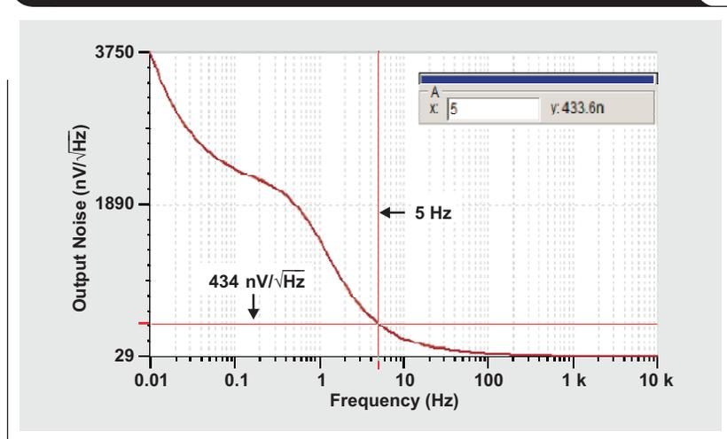
**Figure 14. Simulation of output noise from circuit in Figure 12 with  $R_{FB}$  doubled and  $C_{FB}$  halved**
