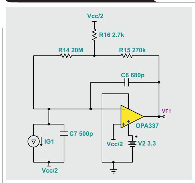
**Figure 16. Improved circuit with differential inputs**
