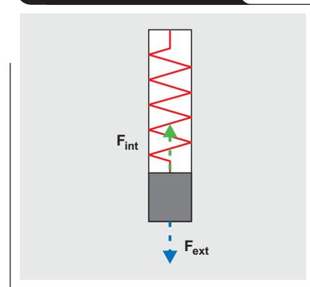
oscillatory force will produce relatively large displacements and therefore large output amplitudes.
