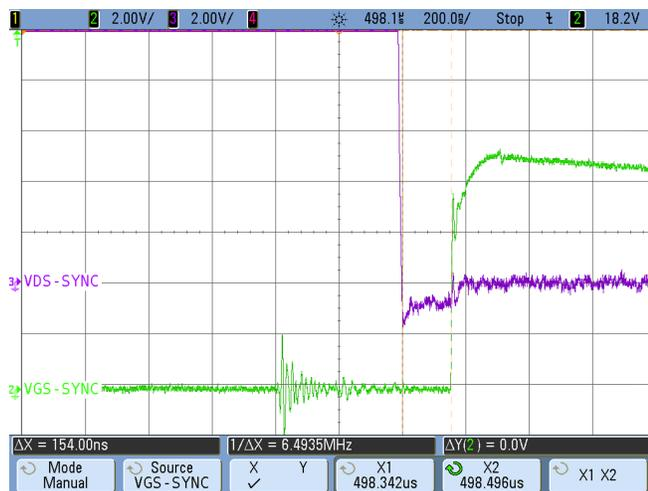
Figure 14. Synchronous MOSFET Turnon
