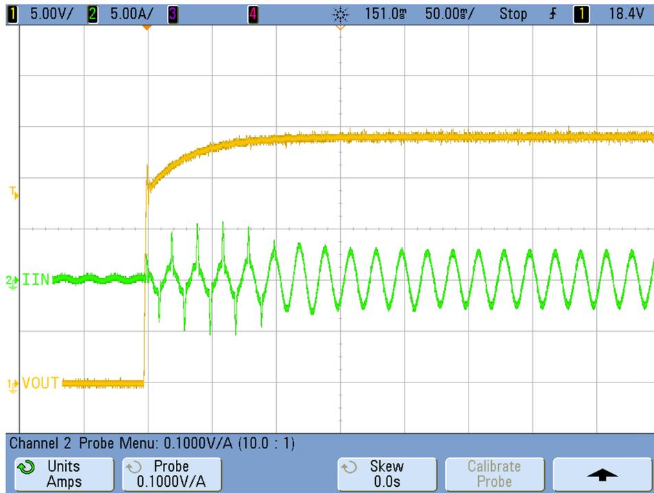
Figure 7. Startup Waveform at 230-V AC
