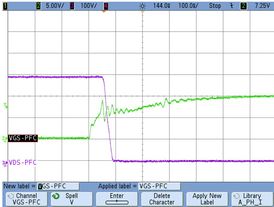
Figure 10. PFC MOSFET Turnon Waveform
