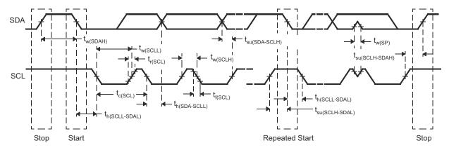
Figure 7-19. I2C Timing Diagram
