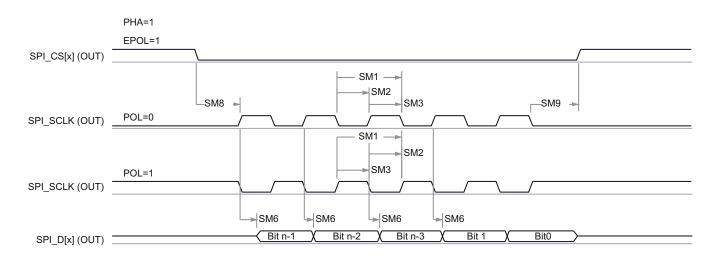
Figure 7-14. SPI Timing- Controller Mode Transmit
