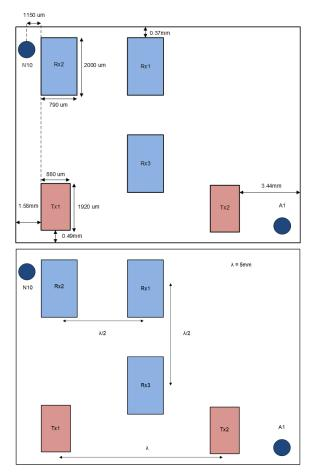
Figure 7-9. Antenna Positions (Placement and Relative Spacing)
