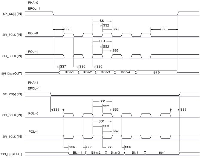
Figure 7-16. SPI Timing - Peripheral mode Transmit
