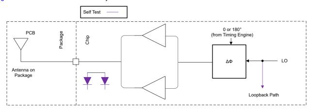
Figure 8-2. Transmit Subsystem (Per Channel)
