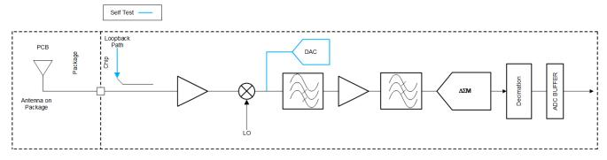
Figure 8-3. Receive Subsystem (Per Channel)
