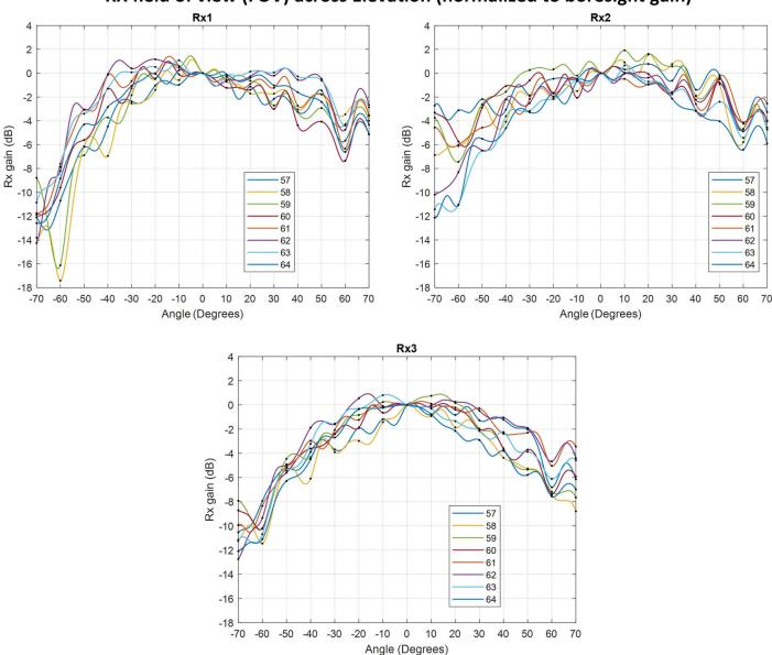
Figure 7-7. Receiver antenna field of view (FOV) normalized to boresight gain
