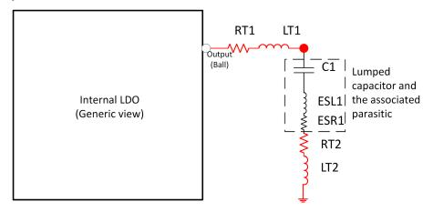
Figure 7-4. Parasitic offered by different portion of the output path (for one capacitor)
