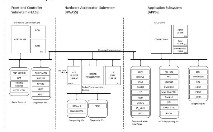
Figure 8-4. Processor Subsystem
