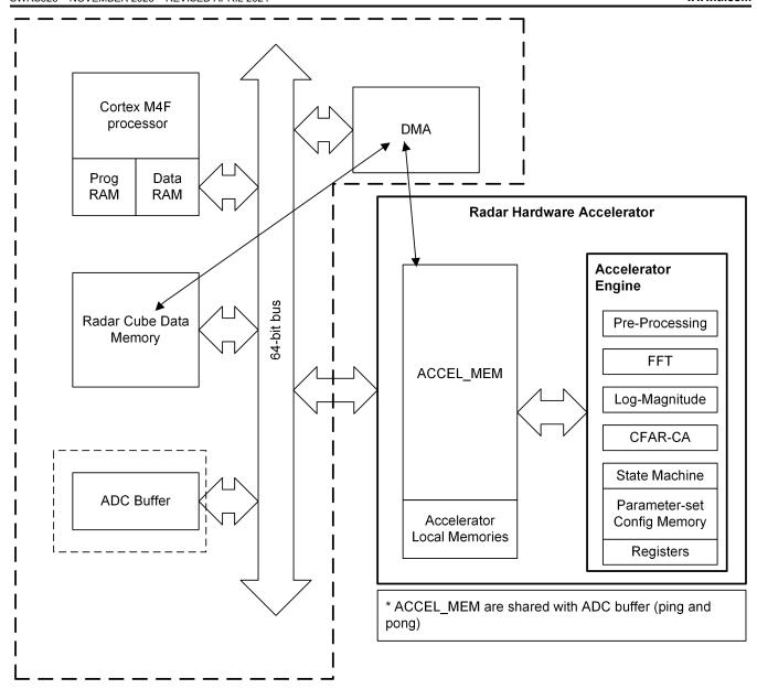
Figure 8-5. HWA 1.2 Functional Block Diagram
