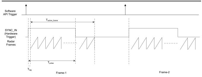
Figure 7-11. Sync In Hardware Trigger
