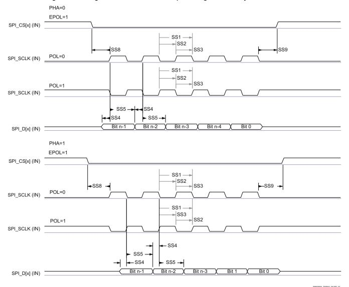
Figure 7-15. SPI Timing - Peripheral mode Receive
