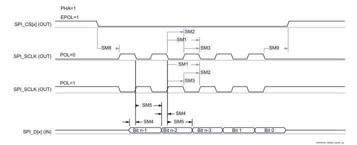
Figure 7-13. SPI Timing -Controller Mode Receive
