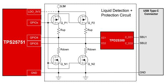
Figure 9-9. TPS25751 Liquid Detection Block Diagram - 1 GPIO Control
