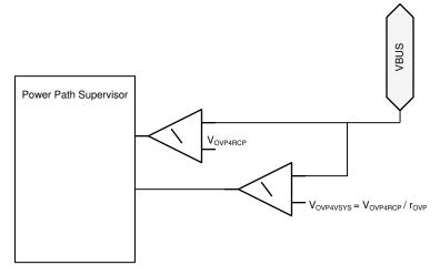
Figure 8-14. Diagram for OVP Comparators
