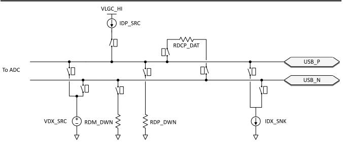
Figure 8-24. BC1.2 Hardware Components
