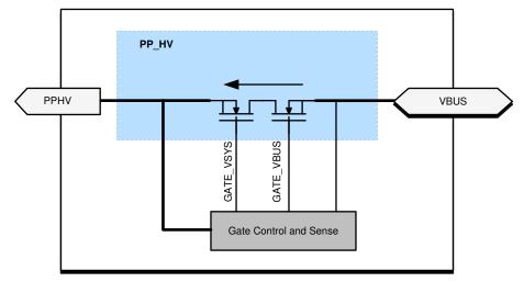
The sink-path control includes overvoltage protection (OVP) and reverse current protection (RCP).
