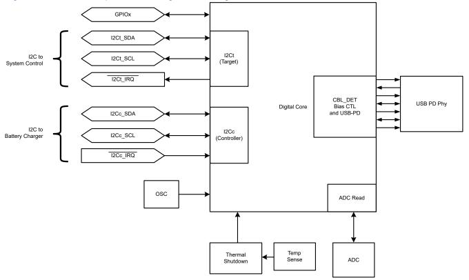
Figure 8-26. Digital Core Block Diagram
