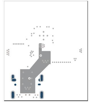
Figure 9-38. TPS25751S PCB Layout - Internal Power Layer
