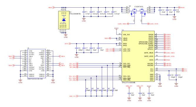
Figure 9-34. TPS25751S Example Schematic
