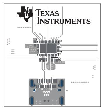
Figure 9-27. TPS25751D PCB Layout - Top Composite
