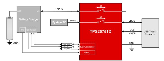
Figure 9-6. TPS25751D PPS with Battery Charger
