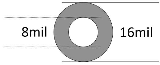
Figure 9-33. Recommend Minimum Via Size
