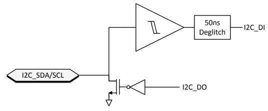
Figure 8-25. I<sup>2</sup>C Buffer
