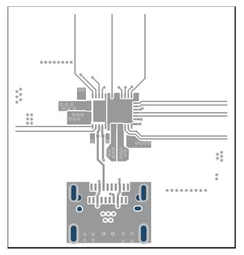
Figure 9-29. TPS25751D PCB Layout - Top Layer Routing
