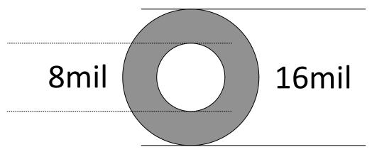
Figure 9-25. Recommend Minimum Via Size
