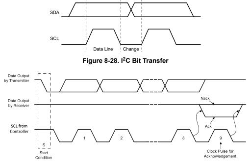
Figure 8-29. I<sup>2</sup>C Acknowledgment
