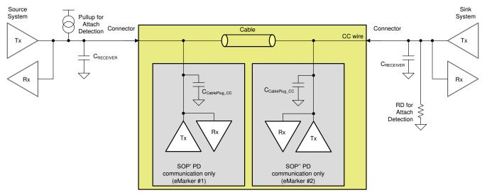
Figure 8-10. Example USB-PD Multi-Drop Configuration
