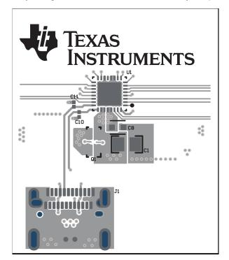
Figure 9-35. TPS25751S PCB Layout - Top Composite
