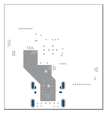
Figure 9-30. TPS25751D PCB Layout - Internal Power Layer
