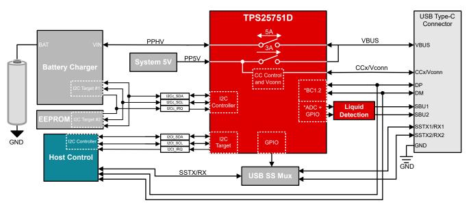
Figure 9-12. TPS25751D USB Data Support
