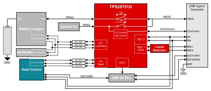
Figure 9-1. TPS25751D Battery Charger & Full System Block Diagram
