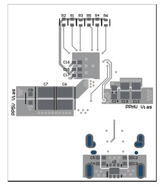
Figure 9-36. TPS25751S PCB Layout - Bottom Composite
