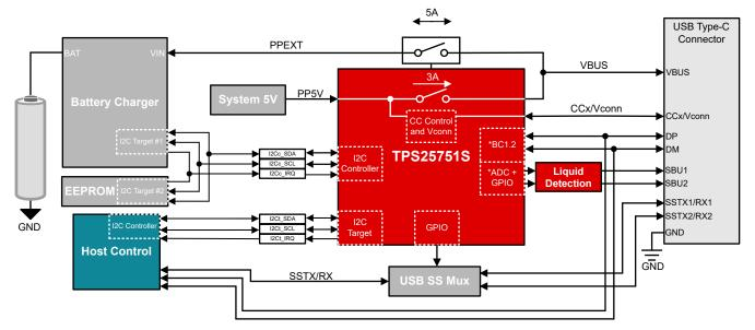
Figure 9-2. TPS25751S Battery Charger & Full System Block Diagram
