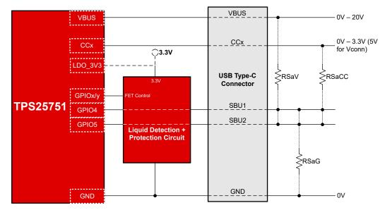
Figure 9-10. TPS25751 Liquid Detection Operation
