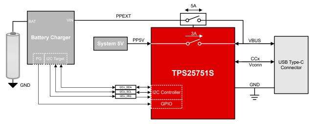
Figure 9-7. TPS25751S PPS with Battery Charger
