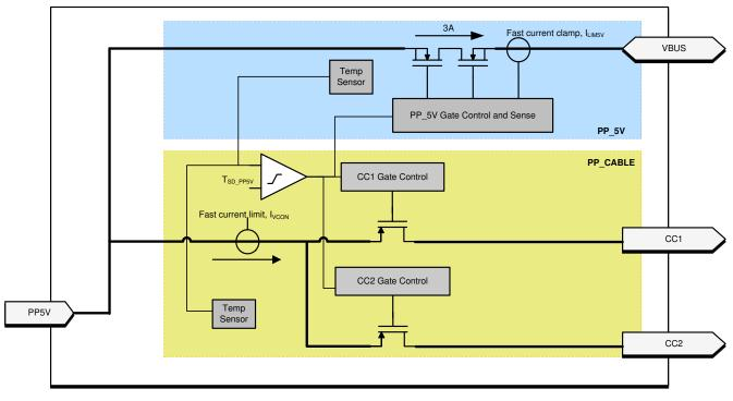
Figure 8-12. Port Power Switches
