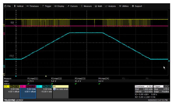
Figure 9-14. PPS PD Negotiation VBUS Increasing/Decreasing
