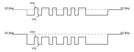
Figure 8-8. TX Driver Transmission with DC Bias
