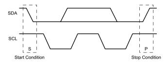
Figure 8-27. I<sup>2</sup>C Definition of Start and Stop Conditions
