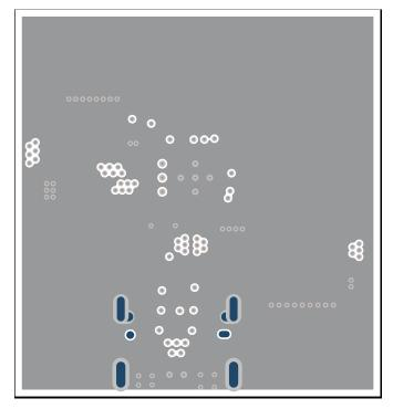
Figure 9-31. TPS25751D PCB Layout - GND Layer
