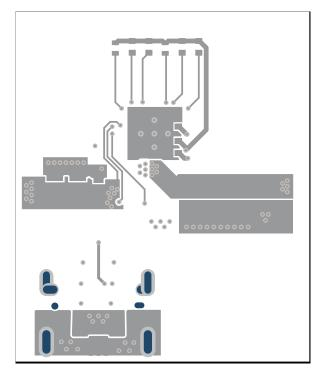
Figure 9-40. TPS25751S PCB Layout - Bottom Layer
