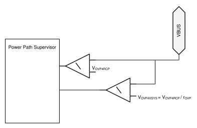
Figure 8-18. Diagram for OVP Comparators
