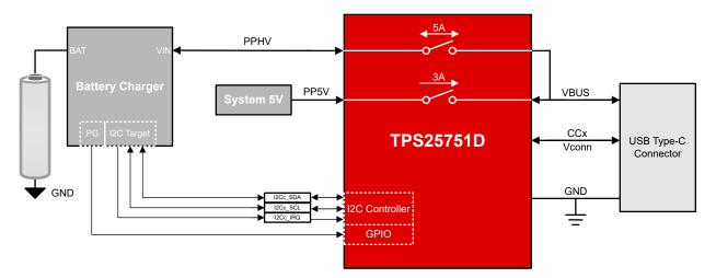
Figure 9-3. TPS25751D Battery Charger System Block Diagram
