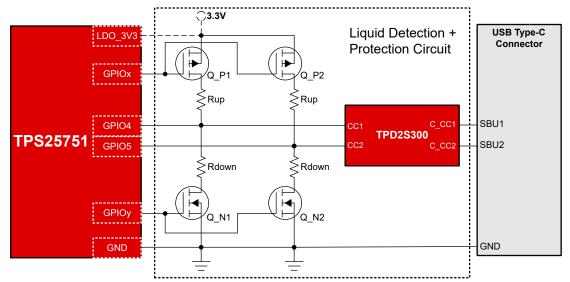
Figure 9-8. TPS25751 Liquid Detection Block Diagram - 2 GPIO Control
