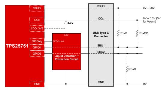
Figure 9-5. Liquid Detection Cases
