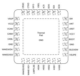
Figure 4-1. RHB Package, 32 Pin (VQFN) (Top View)
