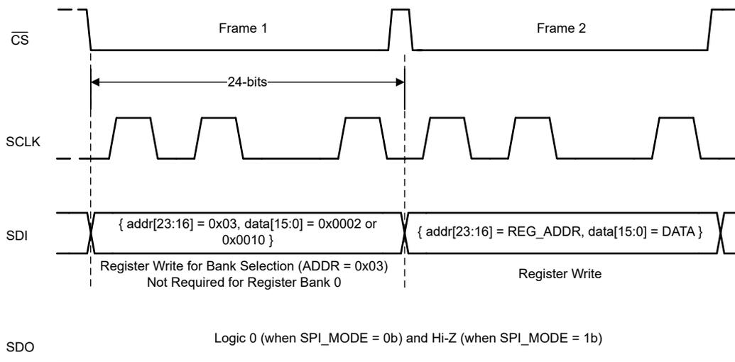
**Figure 6-9. Register Write**
