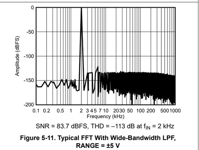
Figure 5-11. Typical FFT With Wide-Bandwidth LPF, RANGE =  $\pm 5\text{ V}$
