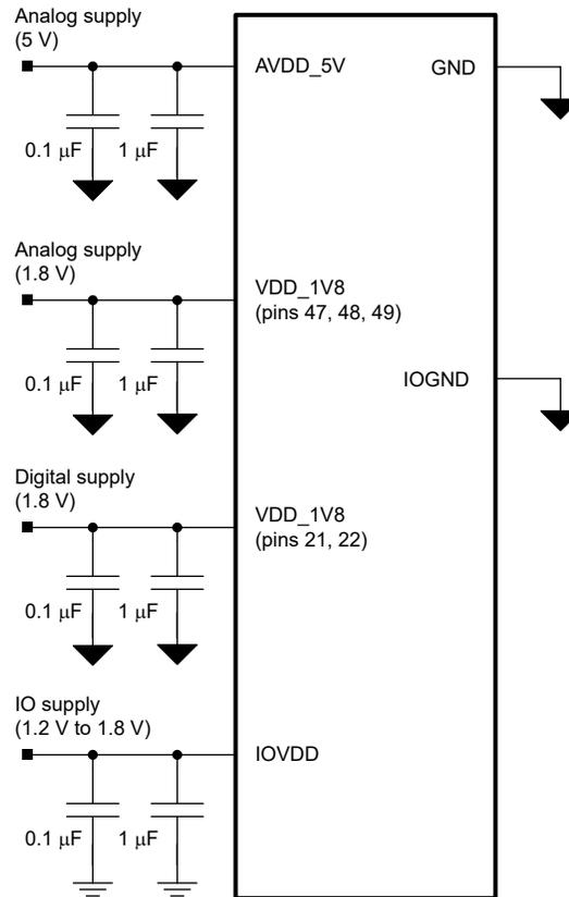
**Figure 8-4. Power-Supply Decoupling**
