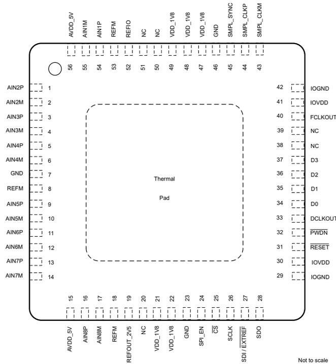
**Figure 4-1. RSH Package, 56-Pin VQFN (Top View)**
