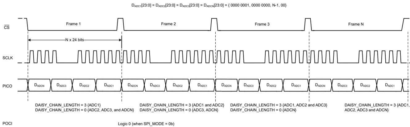
**Figure 6-13. Register Write to Configure Daisy-Chain Length**
