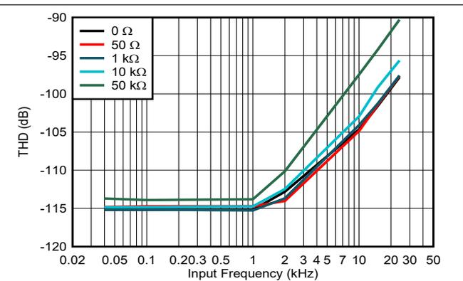
Figure 5-23. THD vs Input Frequency, High-BW Mode, RANGE =  $\pm 5\text{ V}$ , ADS9817
