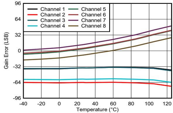
Figure 5-37. Gain Error vs Temperature, RANGE =  $\pm 5\text{ V}$
