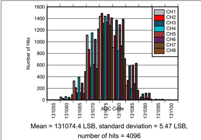
Figure 5-42. DC Histogram of Codes for  $AINxP = AINxM = GND$ , Wide-BW Mode, RANGE =  $\pm 5\text{ V}$
