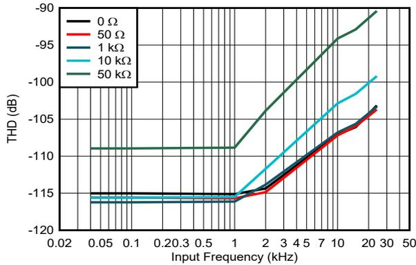
**Figure 5-24. THD vs Input Frequency, Low-BW Mode, RANGE =  $\pm 10\text{ V}$ , ADS9817**
