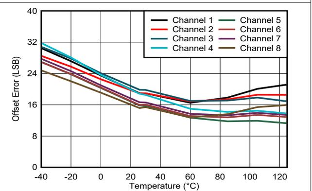
Figure 5-35. Offset Error vs Temperature, RANGE =  $\pm 10\text{ V}$
