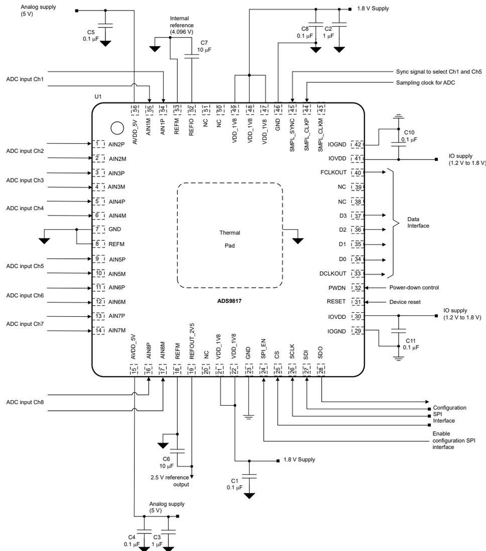
**Figure 8-1. Recommended Schematic**
