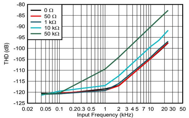
**Figure 5-29. THD vs Input Frequency, High-BW Mode, RANGE =  $\pm 10\text{ V}$ , ADS9815**
