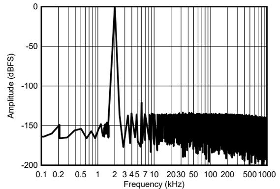
SNR = 85.5 dBFS, THD = -113 dB at  $f_{IN} = 2\text{ kHz}$
