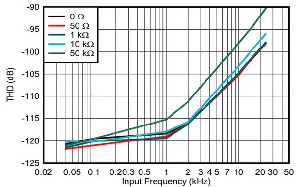
**Figure 5-27. THD vs Input Frequency, High-BW Mode, RANGE =  $\pm 5\text{ V}$ , ADS9815**
