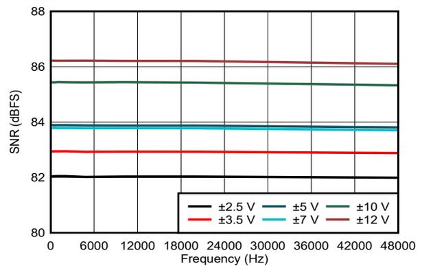
**Figure 5-17. SNR vs Input Signal Frequency Across Input Ranges With Wide-Bandwidth LPF**
