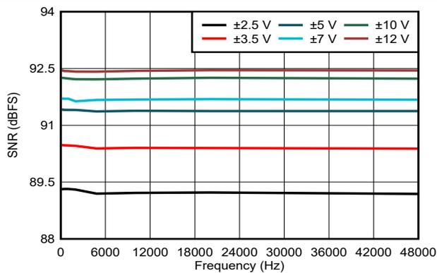
**Figure 5-16. SNR vs Input Signal Frequency Across Input Ranges With Low-Bandwidth LPF**
