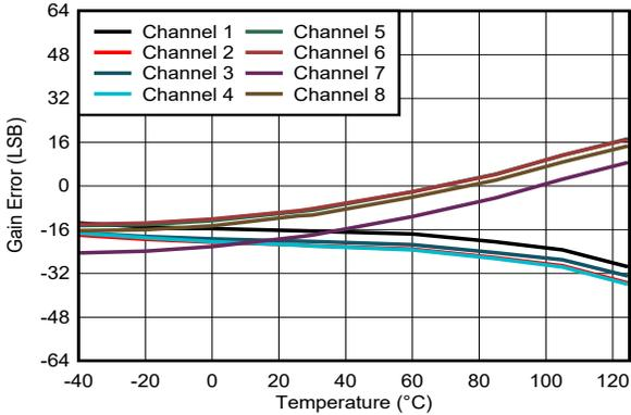
Figure 5-38. Gain Error vs Temperature, RANGE =  $\pm 10\text{ V}$
