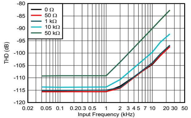
**Figure 5-25. THD vs Input Frequency, High-BW Mode, RANGE =  $\pm 10\text{ V}$ , ADS9817**
