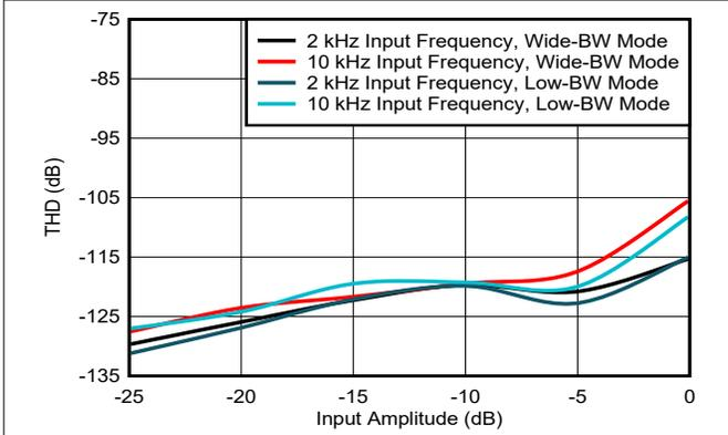
Figure 5-30. THD vs Input Amplitude, RANGE =  $\pm 5\text{ V}$
