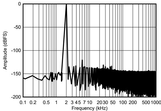
SNR = 92.1 dBFS, THD = -113 dB at  $f_{IN} = 2\text{ kHz}$
