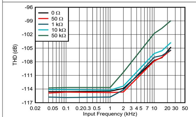
Figure 5-22. THD vs Input Frequency, Low-BW Mode, RANGE =  $\pm 5\text{ V}$ , ADS9817
