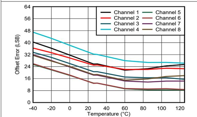
Figure 5-34. Offset Error vs Temperature, RANGE =  $\pm 5\text{ V}$
