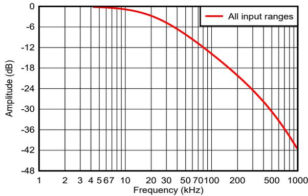
Typical bandwidth ( $-3\text{ dB}$ ) = 21.2 kHz
