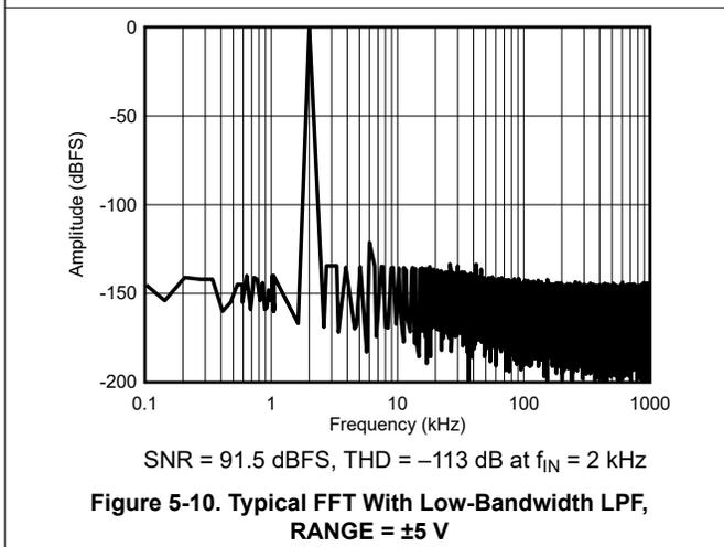
Figure 5-10. Typical FFT With Low-Bandwidth LPF, RANGE =  $\pm 5\text{ V}$
