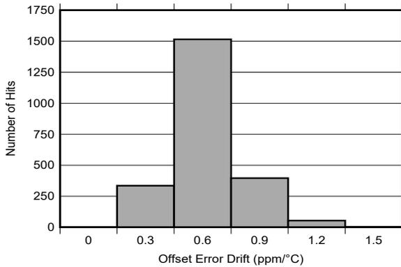
Figure 5-36. Offset Error Drift Histogram
