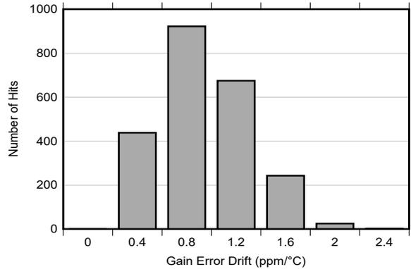
Figure 5-39. Gain Error Drift Histogram
