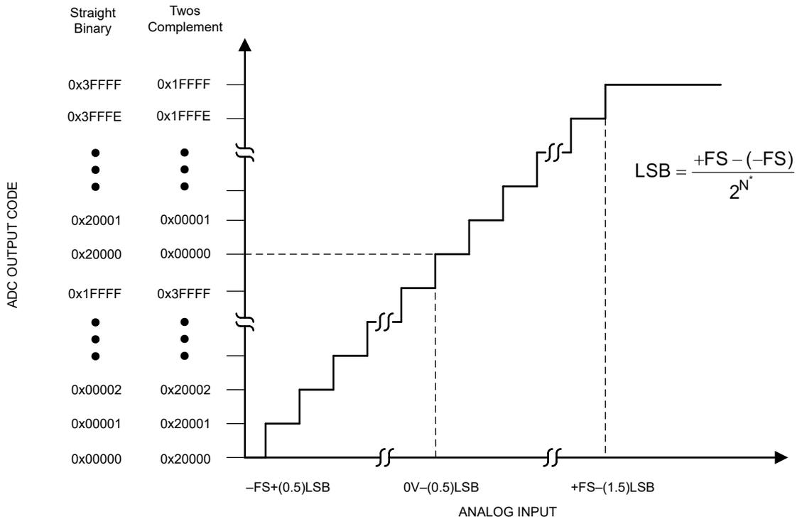
**Figure 6-3. Transfer Characteristics**
