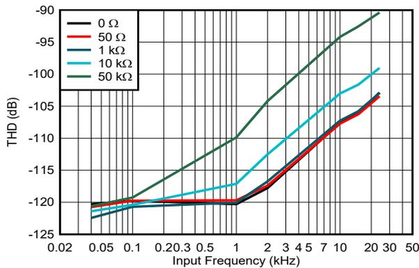
**Figure 5-28. THD vs Input Frequency, Low-BW Mode, RANGE =  $\pm 10\text{ V}$ , ADS9815**
