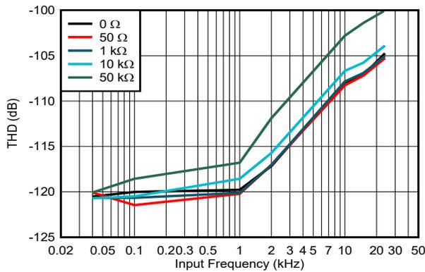
**Figure 5-26. THD vs Input Frequency, Low-BW Mode, RANGE =  $\pm 5\text{ V}$ , ADS9815**
