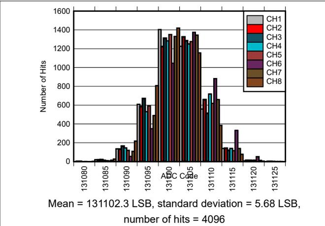
Figure 5-43. DC Histogram of Codes for  $V_{IN} = 1\text{ mV}$ , Wide-BW Mode, RANGE =  $\pm 5\text{ V}$
