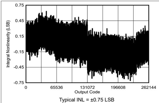
Figure 5-6. Typical INL With Low-Bandwidth LPF
