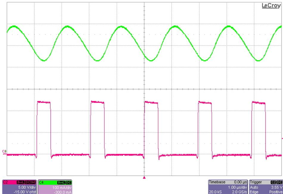
The waveforms below show the switch node voltage (RED) at TP2 and the LED current (GREEN). The input voltage is 18V and the LED output is regulated to 0.5A. (5V/DIV, 100mA/DIV, 1uS/DIV)
