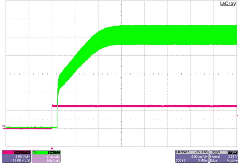
The LED current (GREEN) startup waveform is shown after the input voltage (RED) is applied. The input voltage was set to 12V and the LED current is 0.5A. (5V/DIV, 100mA/DIV, 5mS/DIV)
