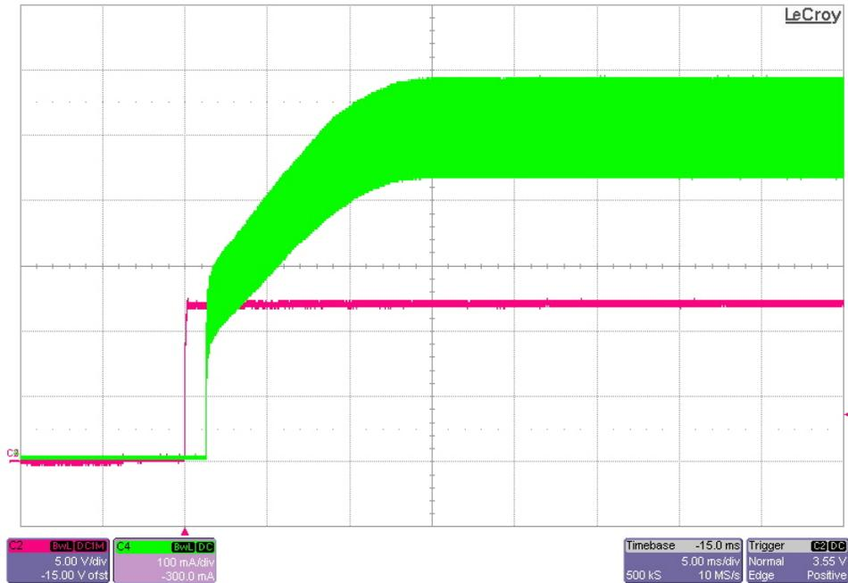
The LED current (GREEN) startup waveform is shown after the input voltage (RED) is applied. The input voltage was set to 18V and the LED current is 0.5A. (5V/DIV, 100mA/DIV, 5mS/DIV)
