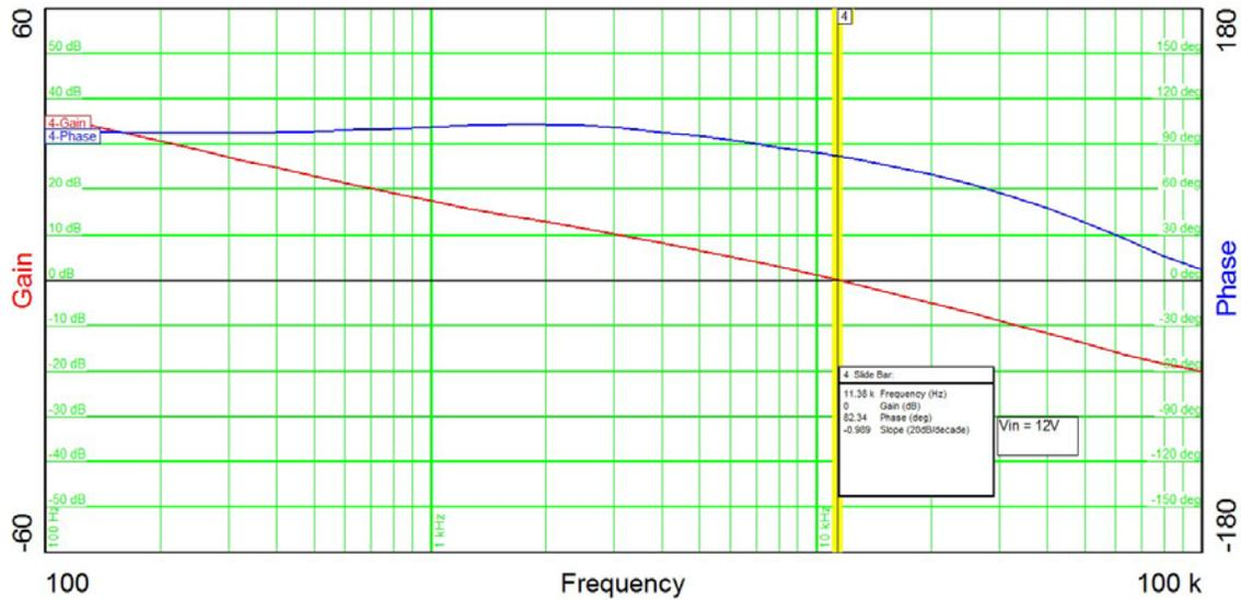
The plot below shows the converter's gain and phase margin for an LED current of 0.5A.
