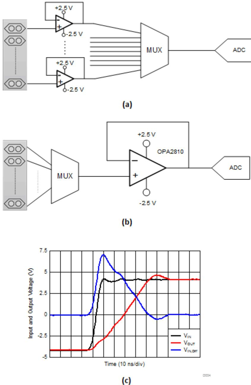
**Figure 4. A Multichannel Sensor Front End with Multiple Slow-settling Amplifiers (a); Using a Single OPA2810 with Fast Settling (b); Large-signal Transient Response Using the OPA2810 (c)**
