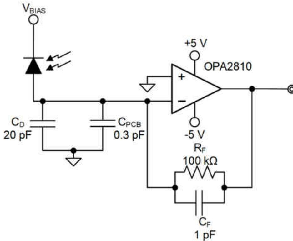
**Figure 2. Photodiode Transimpedance Amplifier Circuit with Feedback Compensation Capacitance**
