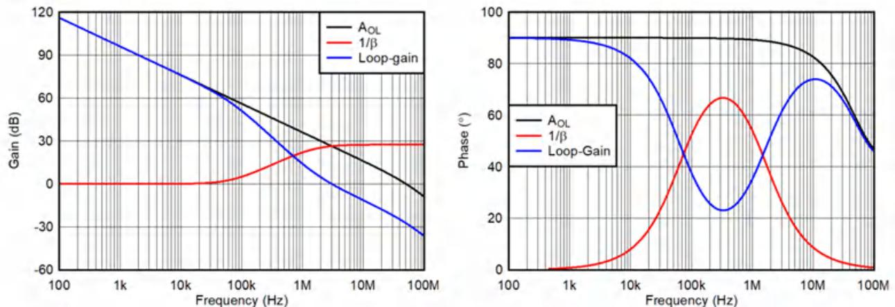
**Figure 3. Gain Magnitude and Phase Bode Plots for the Transimpedance Amplifier in Figure 2**
