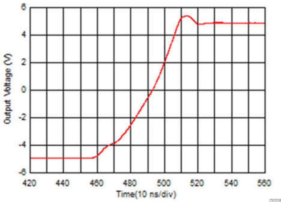
**Figure 5. Large Signal Transient and Settling Response**
