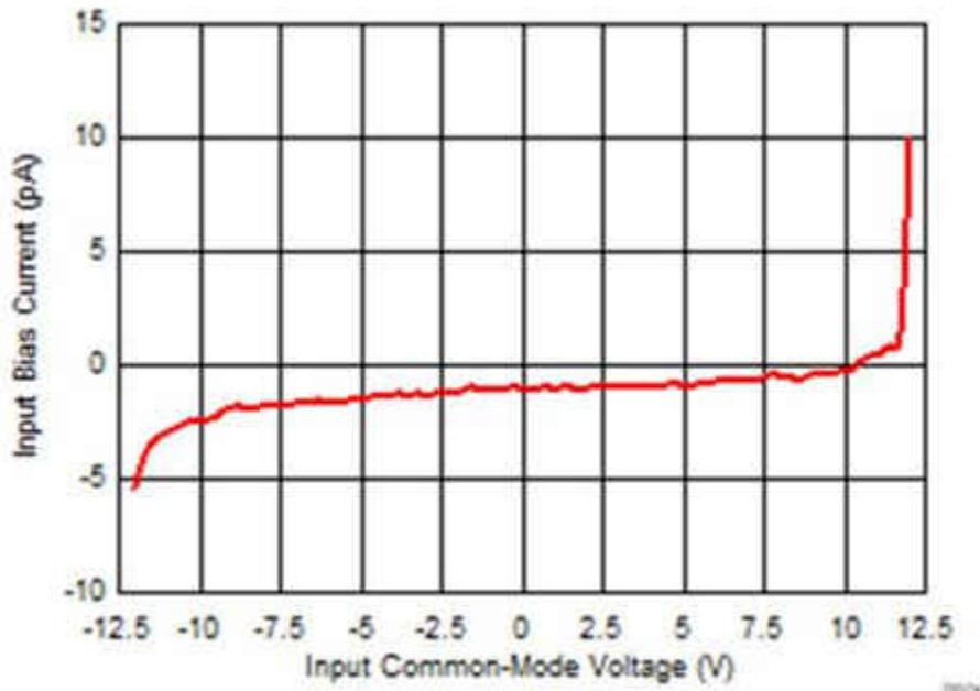
**Figure 1. Bias Current Variation with Input Common-mode Voltage for the OPA2810**
