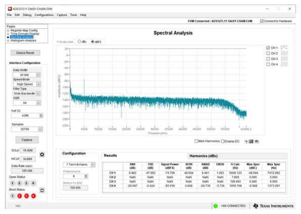
Figure 4-21. Frequency-Domain Plot of 5 kHz Applied to the IEPE Sensor
