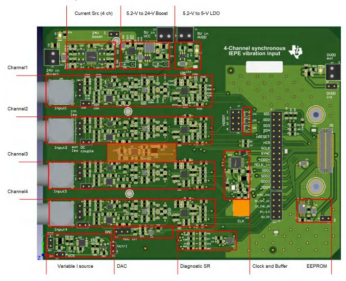
Figure 4-1. PCB Layout
