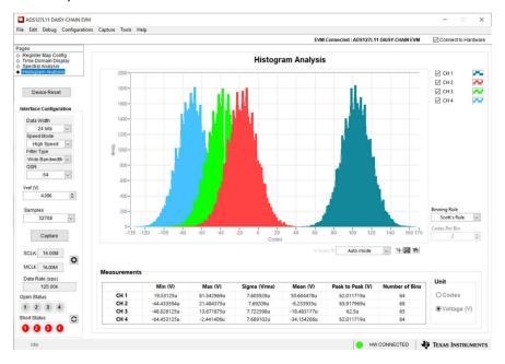
Figure 4-9. Histogram Plot of ADCs Inputs Shorted (Test Mode)
