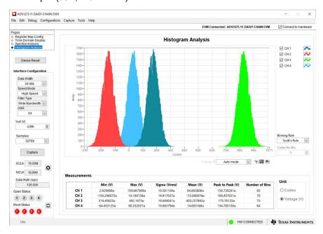
Figure 4-10. Histogram Plot of Front-End Inputs Shorted
