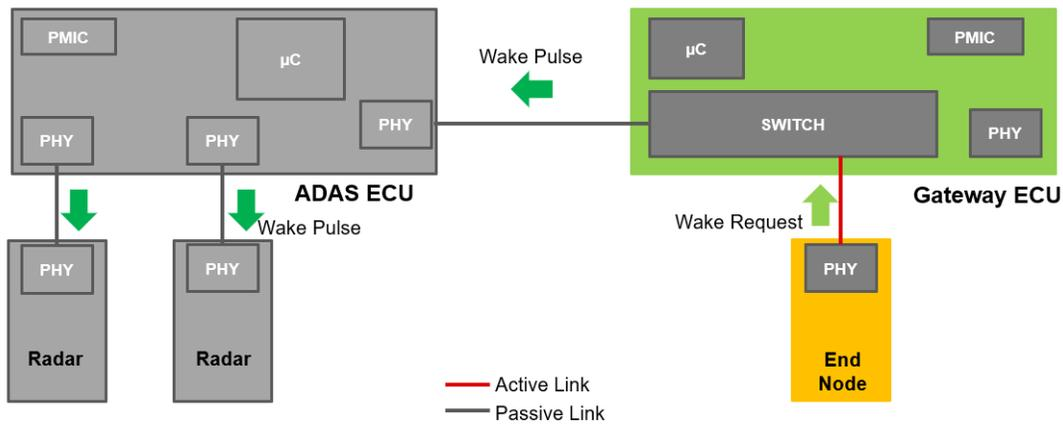
**Figure 5-3. TC10 ADAS System Use Case Example**
