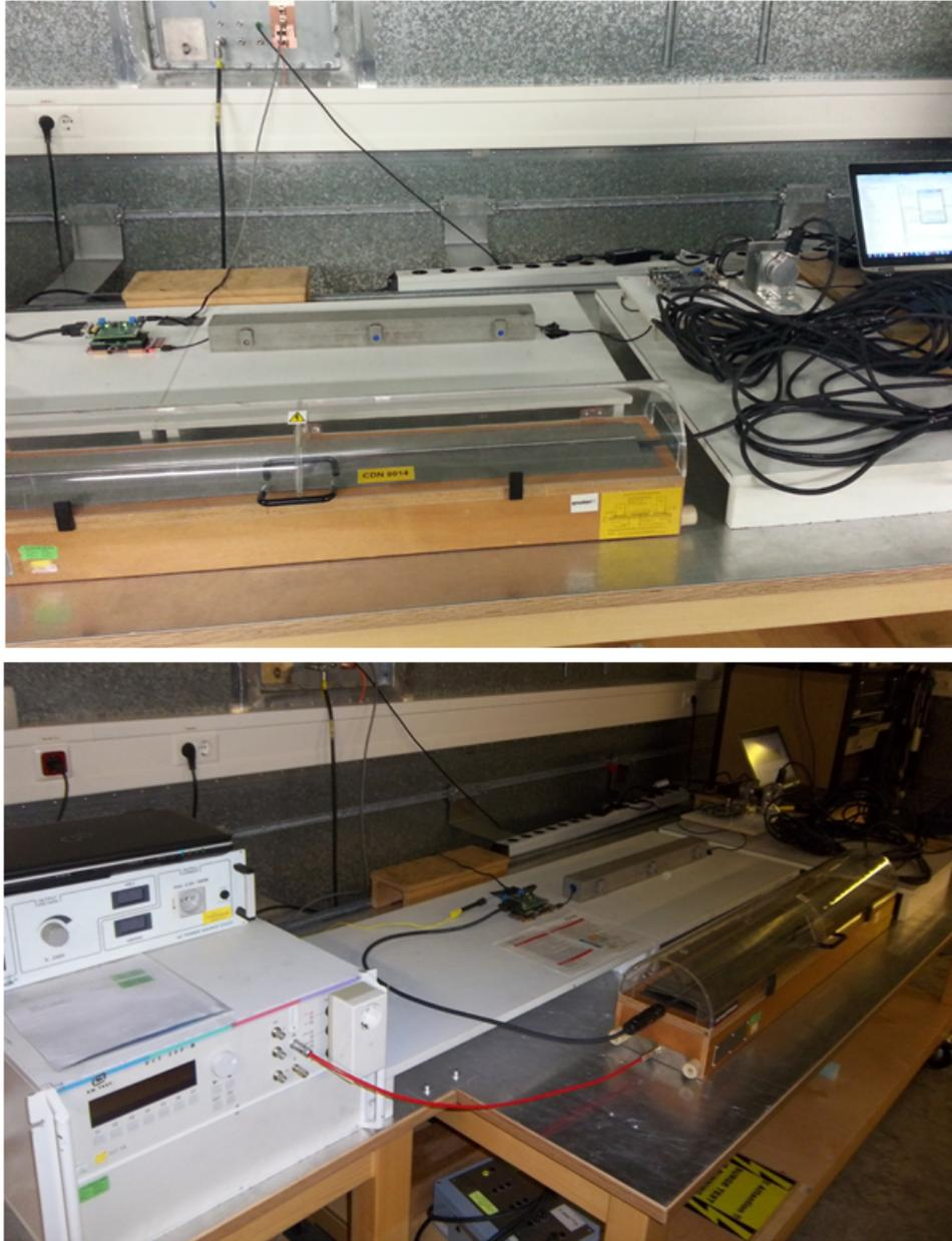
**Figure 75. IEC61000-4-4 EFT Test Setup for TIDA-00176 (Right Side on Top, Left Side on Bottom)**
