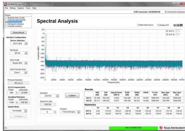
Figure 23. ADC Performance With Gain of 10 at 2 kHz (Same Gain on Both Channels)
