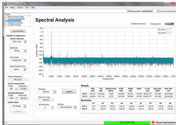
Figure 21. ADC AC Performance With Gain of 10 at 20 kHz (Same Gain on Both Channels)
