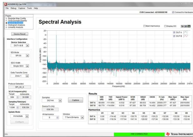
Figure 27. ADC AC Performance With a Gain of 10 at 20 kHz Using 18-Bit ADS8910B
