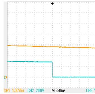
Orange Line (Channel 1) = Power Down Ramp on BAT Pin
