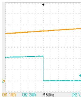
Orange Line (Channel 1) = Power Up Ramp on BAT Pin
