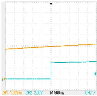
Orange Line (Channel 1) = Power Up Ramp on BAT Pin
