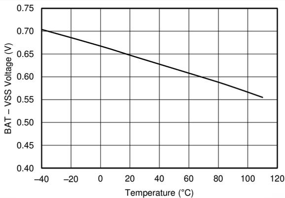
图 6-5. 0V Charging Disallowed Versus Temperature
