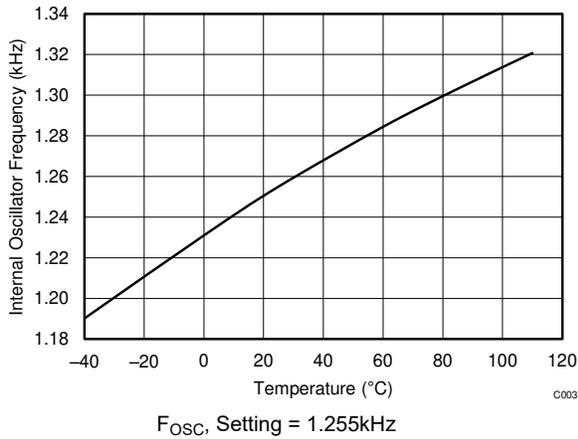
图 6-3. Internal Oscillator Frequency Versus Temperature
