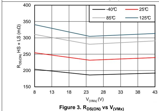
Figure 3.  $R_{DS(ON)}$  vs  $V_{(VMx)}$
