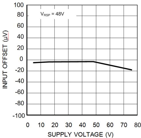
Figure 5. Typical Offset Voltage vs Supply Voltage
