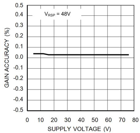
Figure 4. Typical Gain Accuracy vs Supply Voltage
