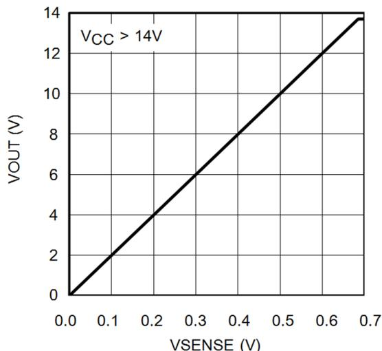
Figure 28. Unidirectional Transfer Function for Gain-of-20 Option
