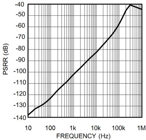
Figure 7. AC Power Supply Rejection Ratio vs Frequency
