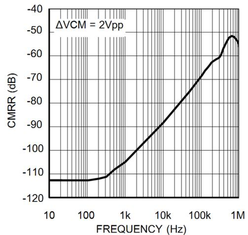
Figure 6. AC Common-Mode Rejection Ratio vs Frequency
