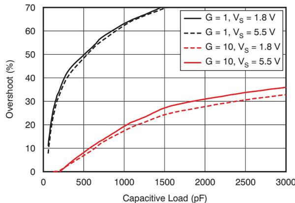
Figure 33. Small-Signal Overshoot versus Capacitive Load (100-mV<sub>PP</sub> output step)
