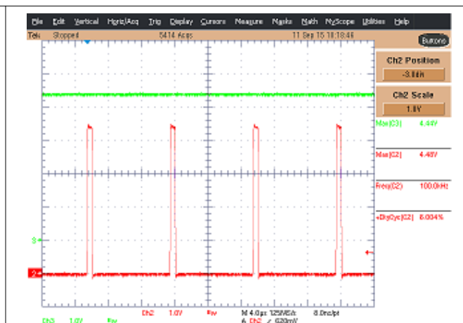
图 8-9. Supply Voltage 5 V Peak Signal 4.5 V
