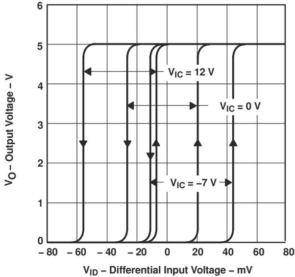
**图 6-9. Receiver Output Voltage vs Differential Input Voltage**
