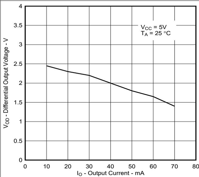
**图 6-3. Driver Differential Output Voltage vs Output Current**
