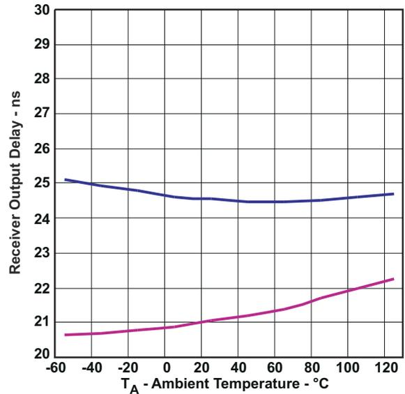
**图 6-12. Receiver Propagation DELAY T<sub>I</sub> vs Free-Air Temperature**
