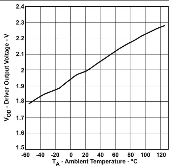
**图 6-4. Driver Differential Output Voltage vs Free-Air Temperature**
