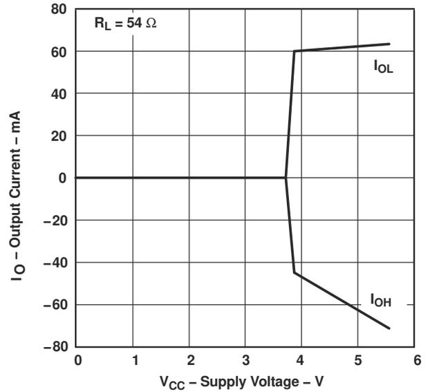
图 6-6. Driver Output Current vs Supply Voltage
