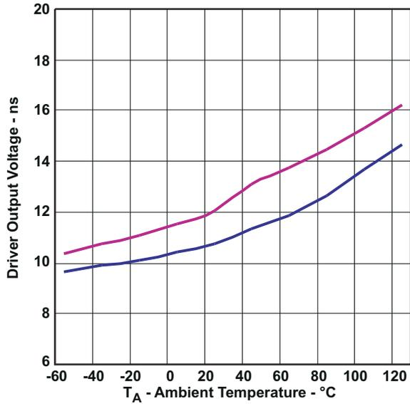
图 6-5. Driver Differential Delay Times vs Free-Air Temperature
