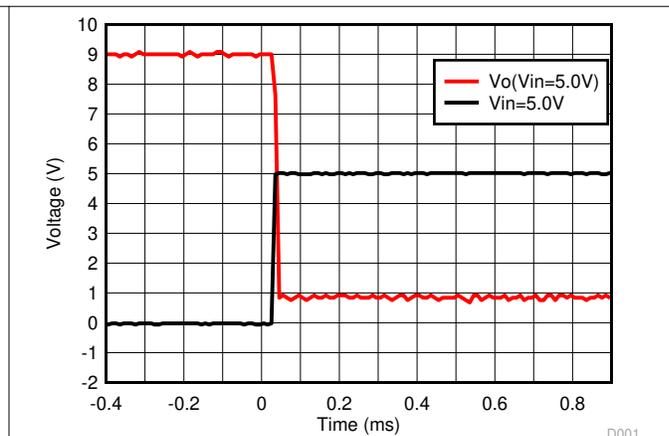
**图 8-4. Output Response With Large Overdrive Voltage**
