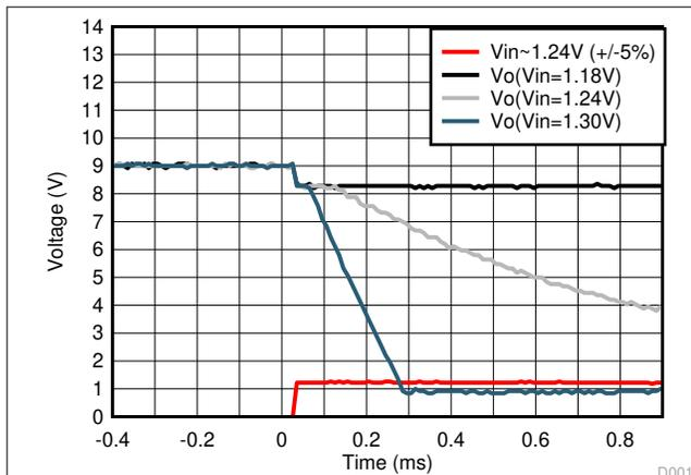
**图 8-3. Output Response With Small Overdrive Voltages**
