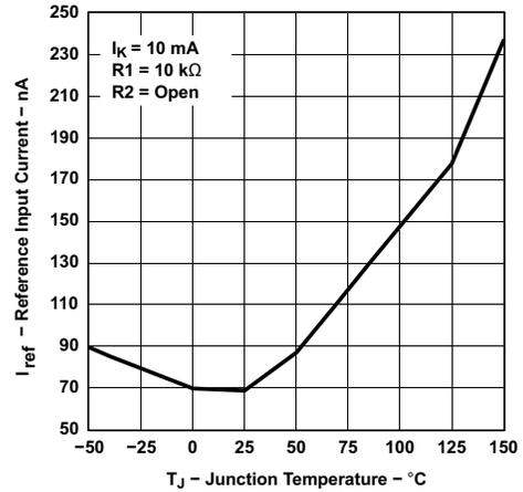
图 5-2. Reference Input Current vs Junction Temperature
