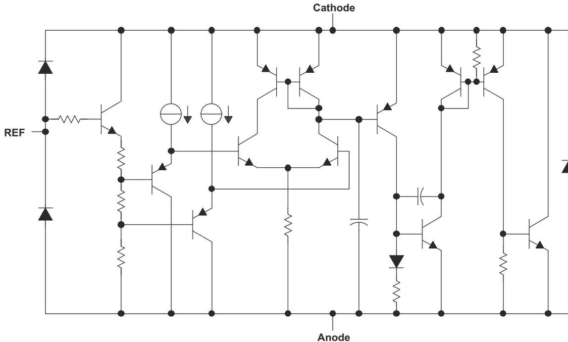
图 7-2. Detailed Schematic
