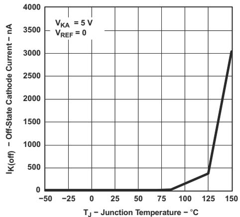
图 5-6. Off-State Cathode Current vs Junction Temperature
