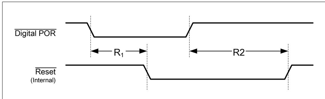
注意: The digital Power-On Reset is only released when the analog Power-On Reset has de-asserted and all of the Power-OK monitors for each of the supplies indicate that power levels are in operational ranges.
