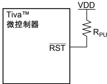
$R_{PU} = 0$  至  $100\text{ k}\Omega$
