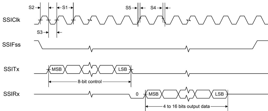
图 22-21. Master Mode SSI Timing for SPI Frame Format (FRF=00), with SPH=1
