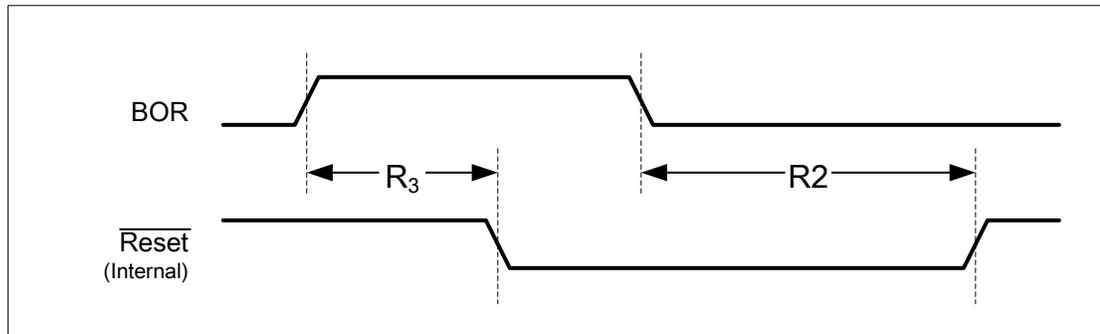
图 22-11. External Reset Timing ( $\overline{\text{RST}}$ )
