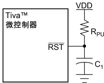
$R_{PU} = 1\text{ k}\Omega$  至  $100\text{ k}\Omega$
