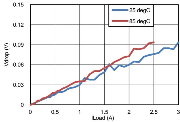
**Figure 16. Vdrop vs ILoad; VGS<sub>Q1</sub> = -7V**
