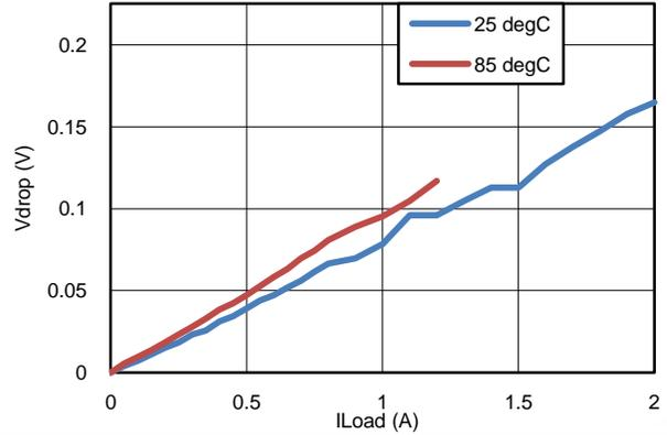
Figure 11. Vdrop vs IL; VGS<sub>Q1</sub>=-1.8V
