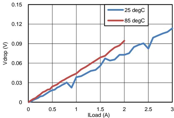
Figure 14. Vdrop vs IL; VGS<sub>Q1</sub>=-4.5V
