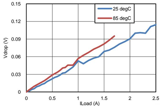
Figure 13. Vdrop vs IL; VGS<sub>Q1</sub>=-3.3V
