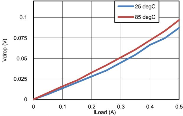
Figure 10. Vdrop vs IL; VGS<sub>Q1</sub>=-1.2V
