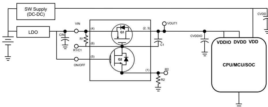
Figure 7. Power Sequencing Using TPS27081A, Example 1
