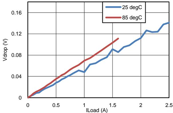
Figure 12. Vdrop vs IL; VGS<sub>Q1</sub>=-2.5V
