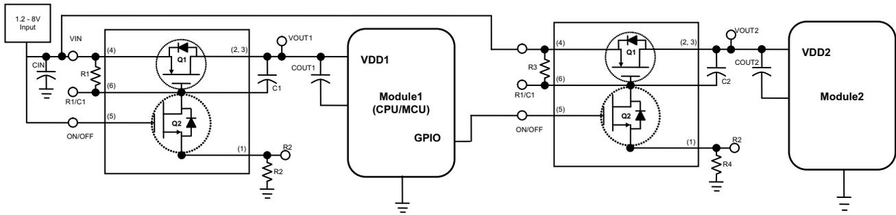
**Figure 8. Power Sequencing Using TPS27081A, Example 2**
