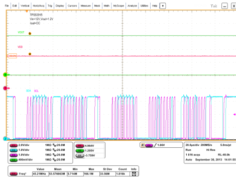
图 32. I 2 C READ (Address=31d, Cmd=0x79): ACK 0x10C8. Ioc = 15 A
