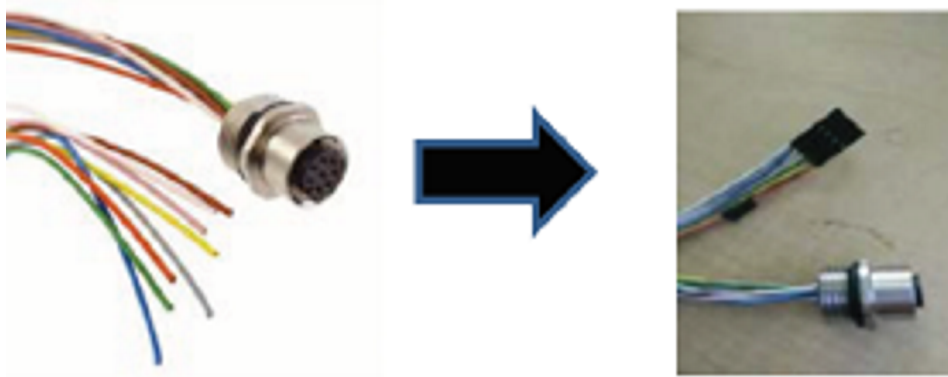
图 10. Adapter to Connect Heidenhain Cable to TIDM-1008 Board
