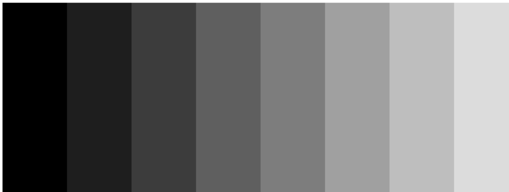
Figure 3-2. Example of Fixed Step Horizontal Ramp Test Pattern
