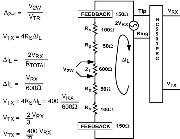
FIGURE 4. TRANSMIT GAIN ACROSS HC5503PRC ( $V_{2W}$  to  $V_{TX}$ )
