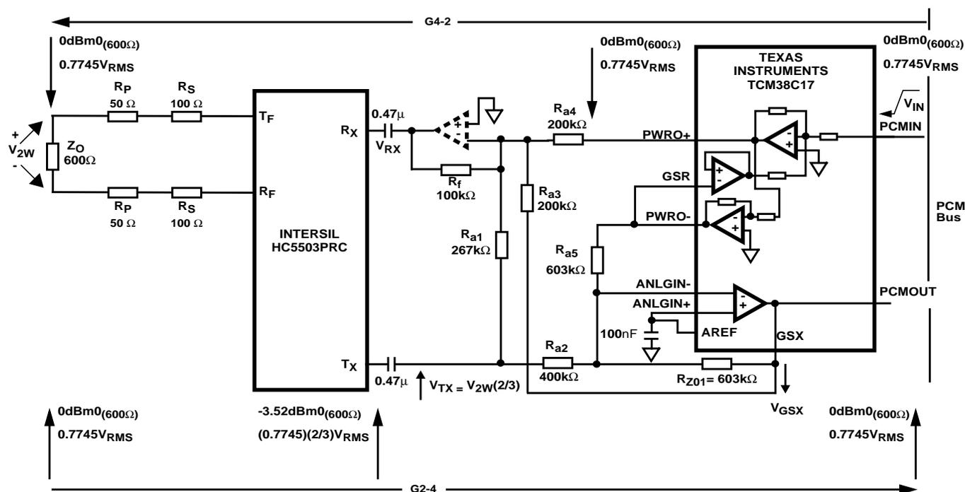
FIGURE 6. Reference Design of the HC5503PRC and the TCM38C17 with a 600Ω Load Impedance
