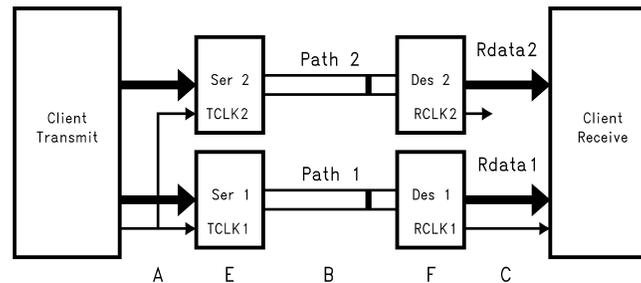
**Figure 1. Parallel Serializers and Deserializers**
