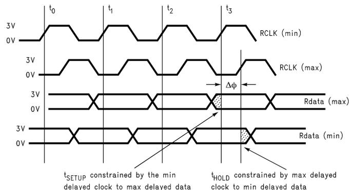
**Figure 2. RCLK and Rdata Timing**
