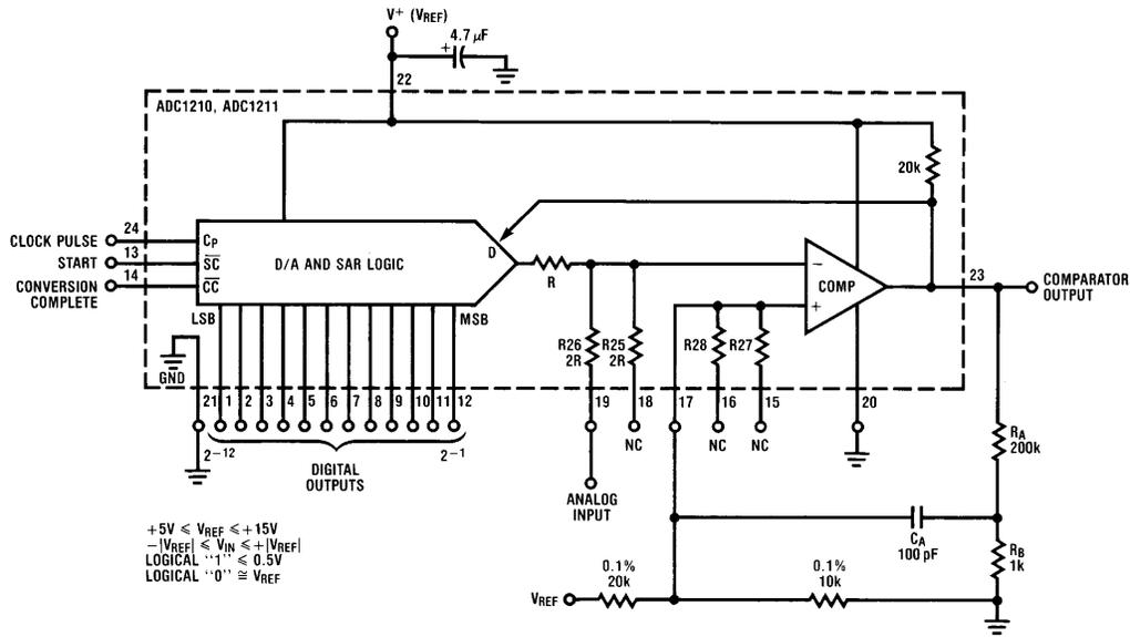
FIGURE 3. Complementary Logic, Bipolar  $-V_{REF}$  to  $+V_{REF}$  Input
