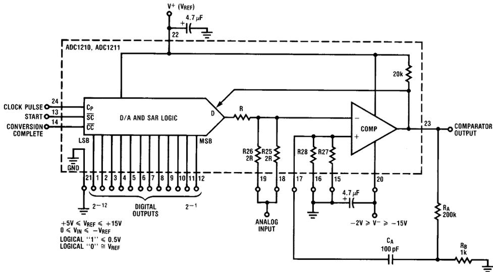
FIGURE 2. Complementary Logic, 0V to  $-V_{REF}$  Input
