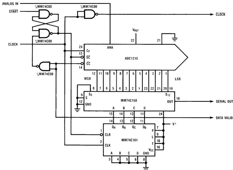
FIGURE 9. 12-Bit A/D Converter with Serial Output
