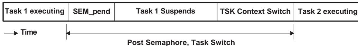
**Figure 16. Pend on Semaphore with Task Switch**
