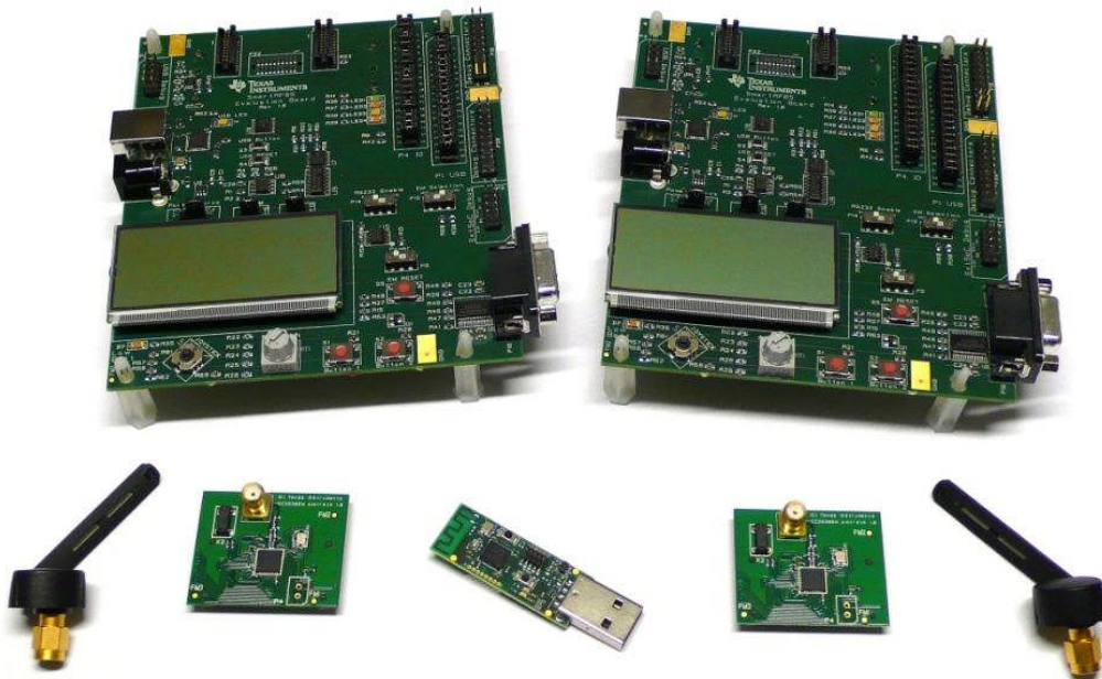
Figure 1 - CC2530 Development Kit Contents
