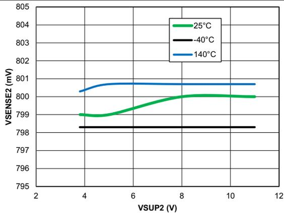
Figure 5. Open-Load Line Regulation BUCK2 = 3.3 V
