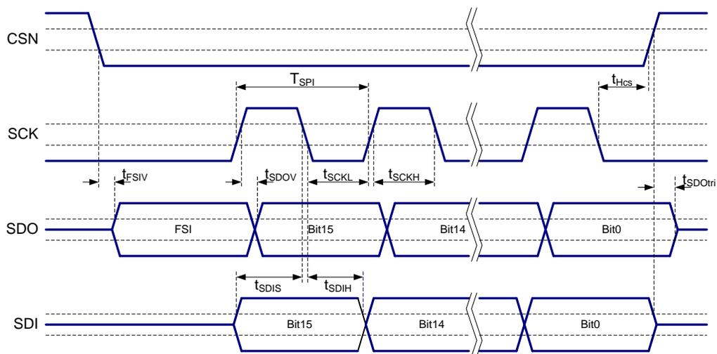
Figure 1. SPI Timing
