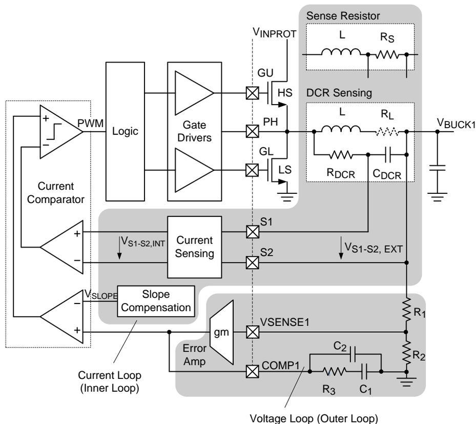
Figure 16. Detailed Block Diagram of Buck 1 Controller
