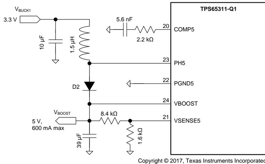
**Figure 35. BOOST Converter Schematic**
