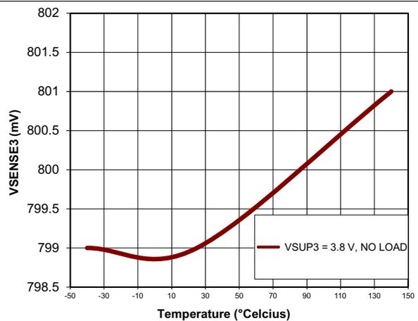
Figure 10. BUCK3 = 1.2-V VSENSE3 vs Temperature
