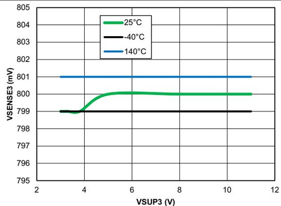
Figure 6. Open-Load Line Regulation BUCK3 = 1.2 V
