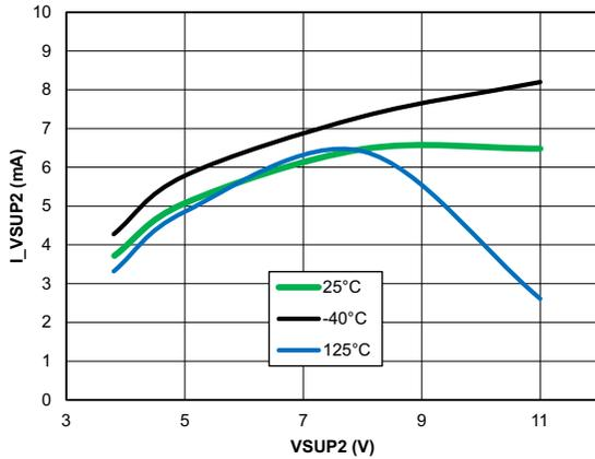
Figure 7. Open-Load Supply Current BUCK2 = 3.3 V
