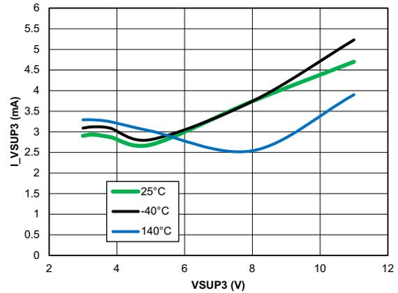
Figure 8. Open-Load Supply Current BUCK3 = 1.2 V
