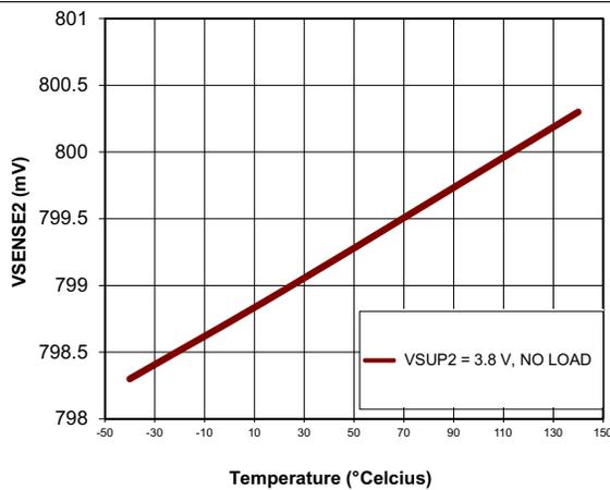
Figure 9. BUCK2 = 3.3-V VSENSE2 vs Temperature
