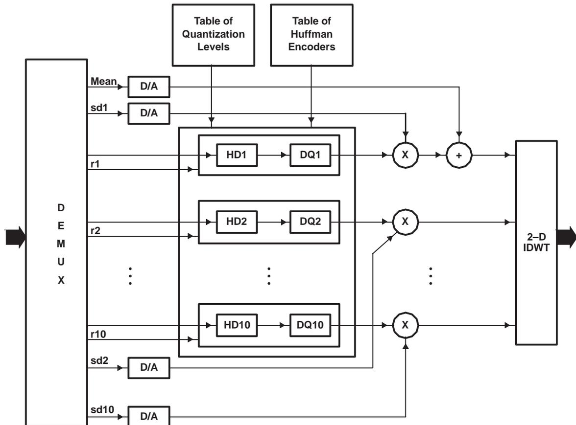
Figure 2. Block Diagram of the Decoder
