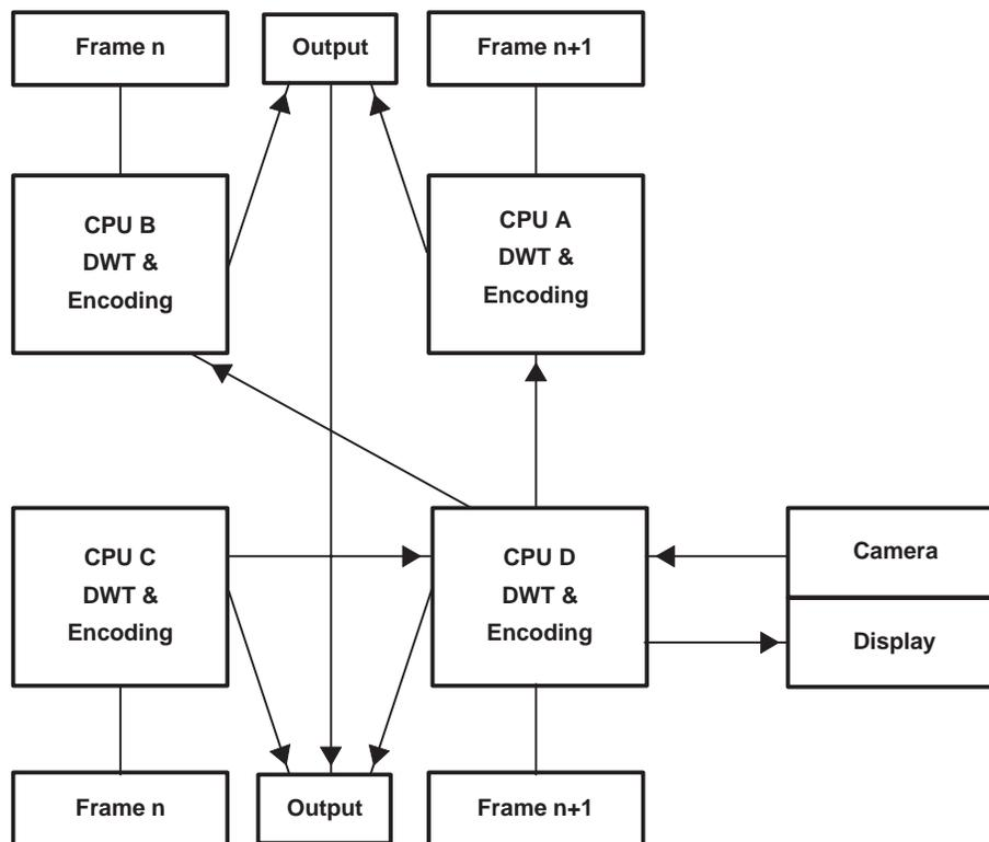
**Figure 5. Hardware Diagram**
