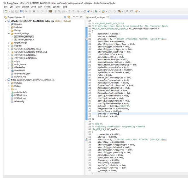
Figure 7-10. Modifying the smartrf\_settings.c File
