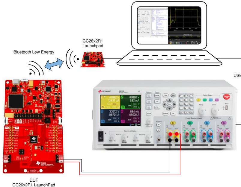
**Figure 6-2. DUT Test Setup**
