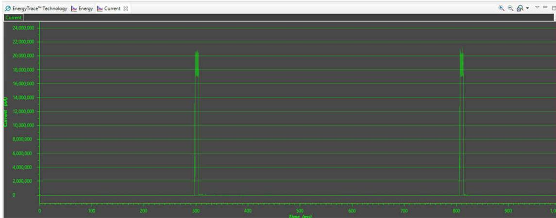
**Figure 7-8. Current Profile for rfPacketTx (without modifications)**
