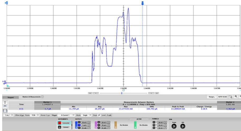
Figure 6-15. Connection Event, Marker #1 Placement
