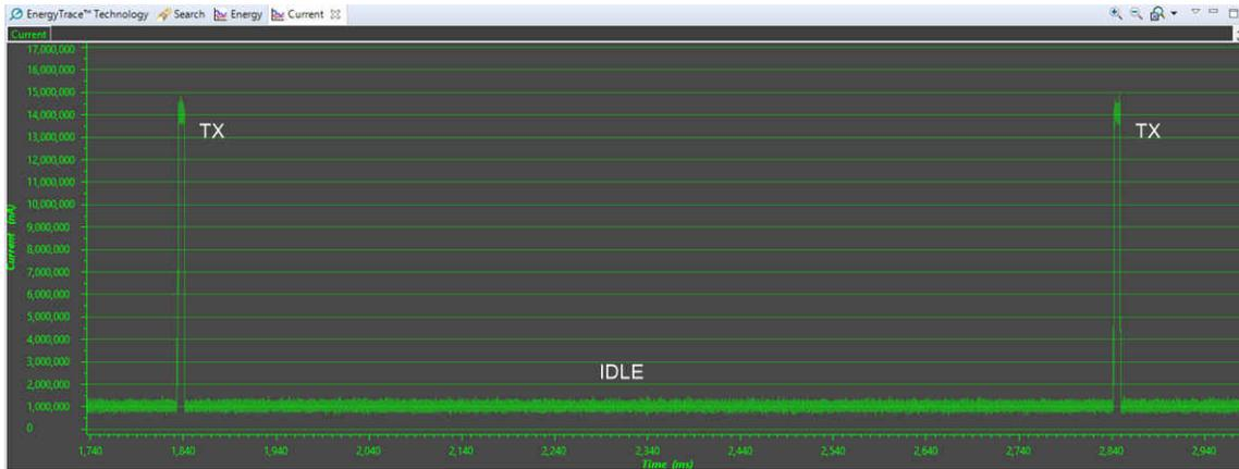
**Figure 7-15. IDLE State Between Packets**
