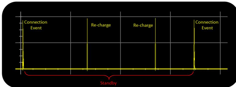
**Figure 3-1. Current Consumption vs. Time During a Bluetooth Low Energy Connection**
