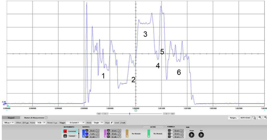
**Figure 6-17. Current Consumption versus Time During a Single Connection Event**
