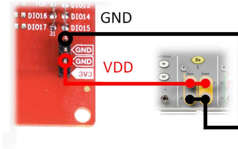
**Figure 6-7. Connecting to the CC26x2r1 LaunchPad**
