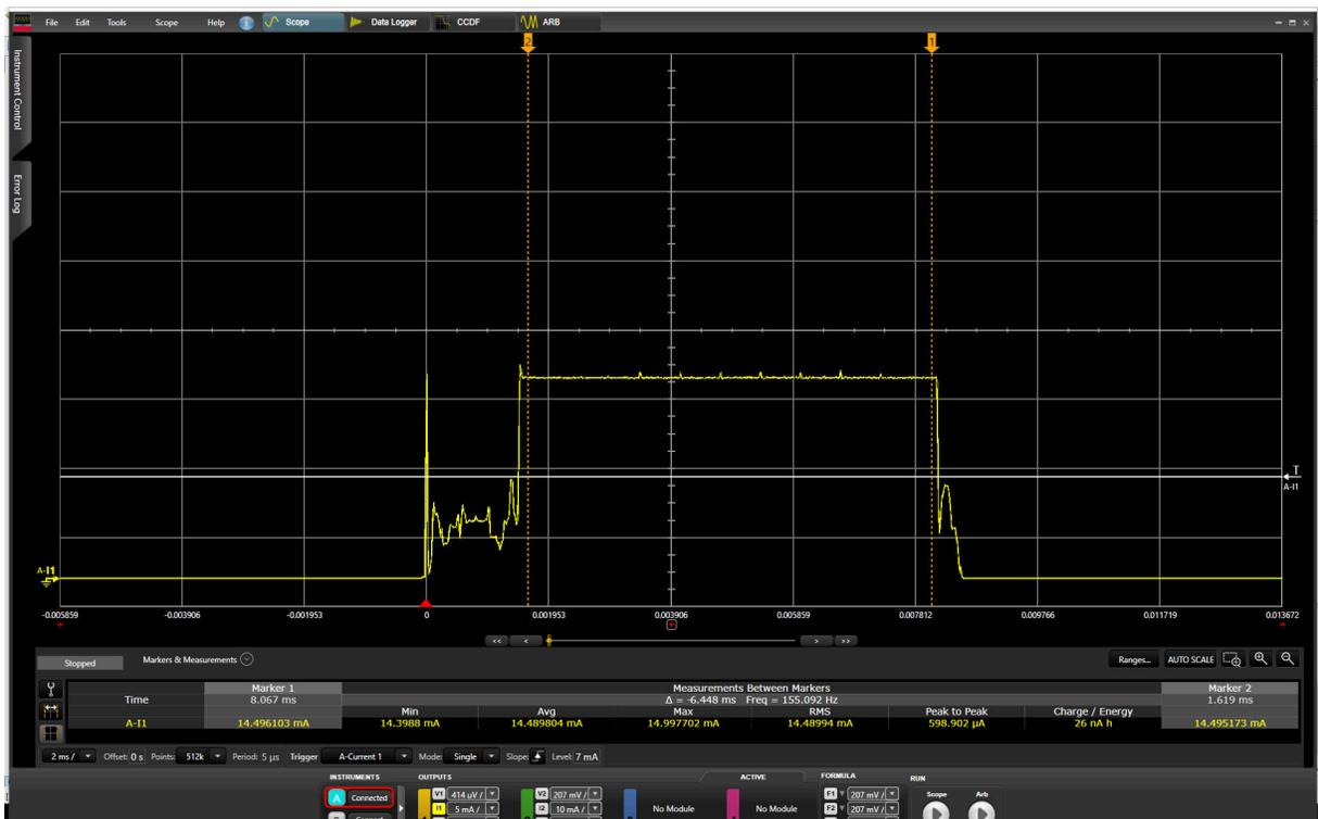
Figure 7-12. Current Profile of TX (DC Power Analyzer)
