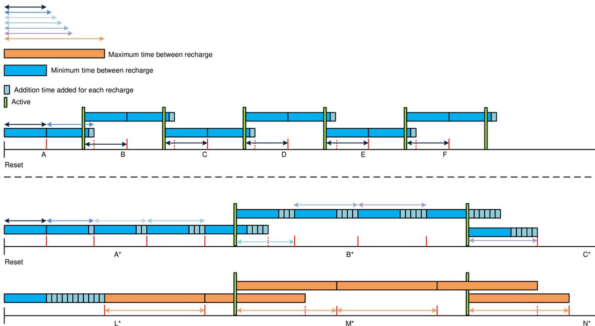
Figure 2-2. Change of Recharge Interval Based on Standby Interval and Time From Reset
