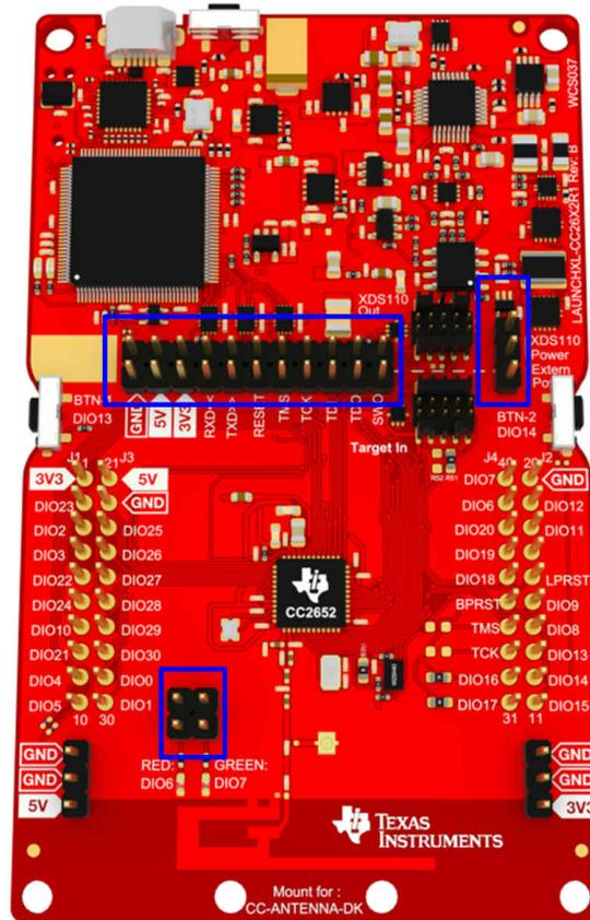
**Figure 5-2. CC2652R LaunchPad Jumper Removal**
