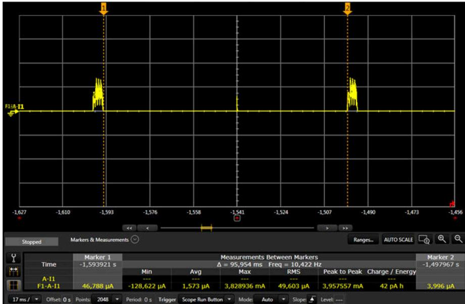
Figure 2-3. Measuring Standby Current During Advertisement (CC26x0)
