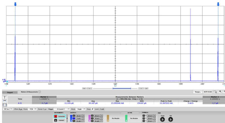
Figure 6-16. Average Current Consumption After Establishing a Connection
