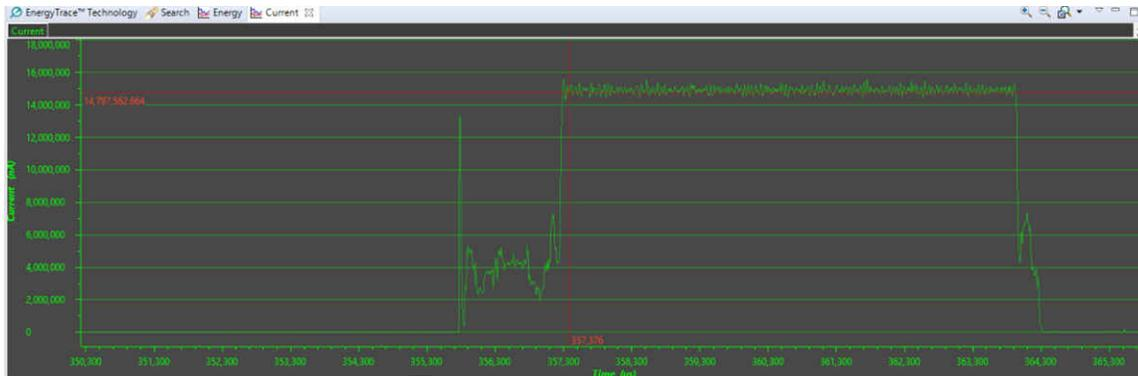
Figure 7-11. Current Profile of TX (EnergyTrace)
