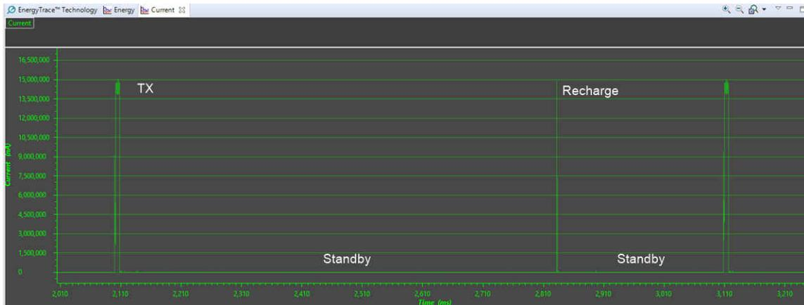
**Figure 7-13. Recharge Pulses**
