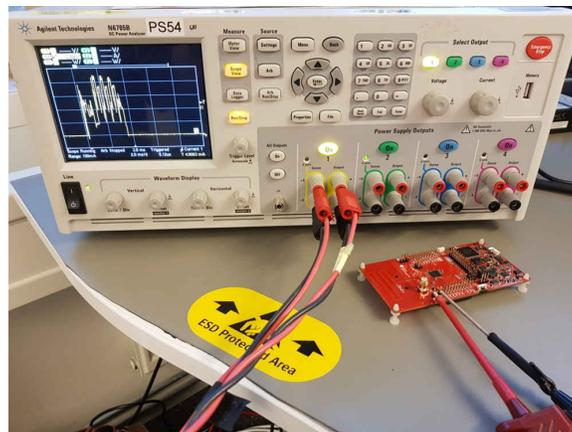
**Figure 6-8. Connected DUT to Agilent 14585A**
