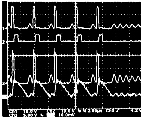
CH1: HDRV, CH2: LDRV, CH3: SW, CH4: I_L (0.2A/div) Output 1V @ 0.04A, VIN = 10V, SKIP, L = 10 \mu H, f = 300kHz
